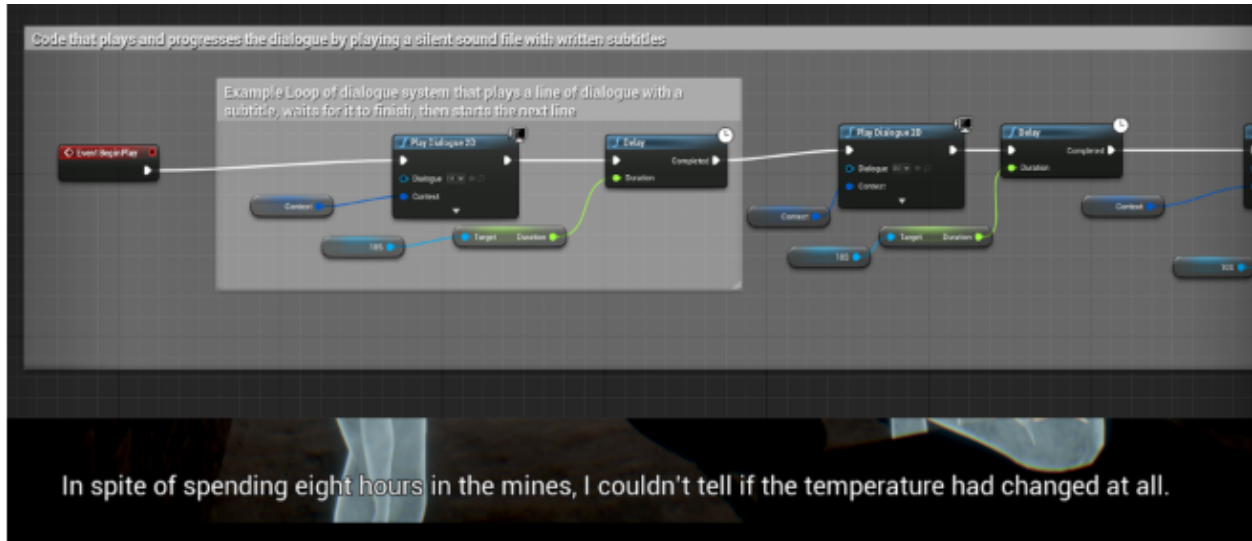
Figure 23: Blueprint for dialogue and underneath is what the blueprint produces
