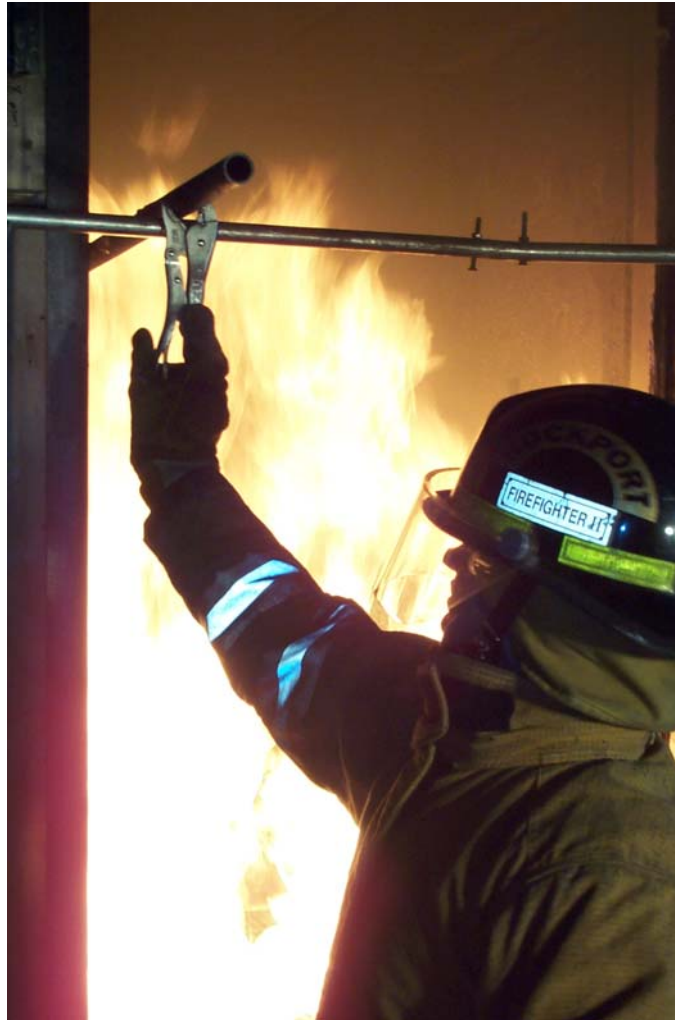
Figure 3-14: Thermocouple tree in the process of being repositioned during testing
