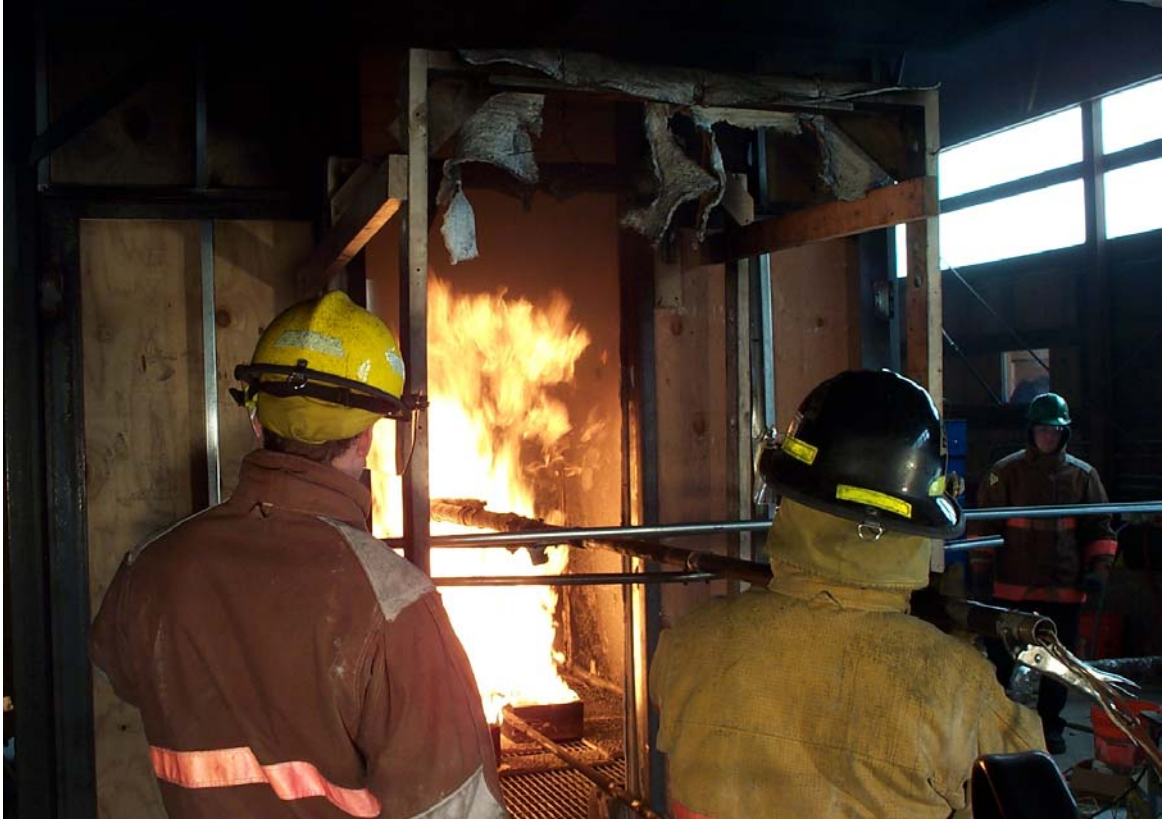
Figure 3-10: Operators collecting flux measurements
