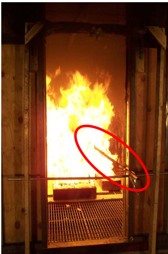
Figure 3-12: Thermocouple tree during testing
