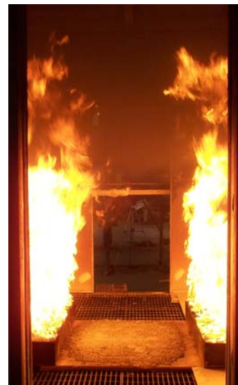
Figure 4-14: Burner configuration B fire conditions
