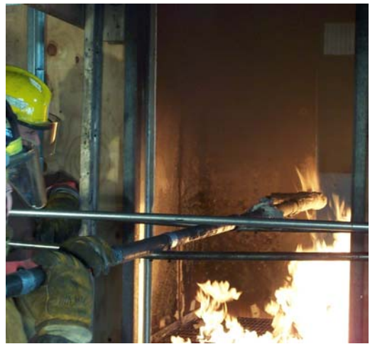
Figure 3-7: Flux gage support and protective structure
