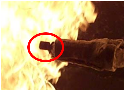
Figure 3-9: The red circle indicates the exposed part of the Schmidt-Boelter gage
