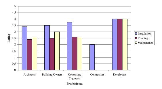
Figure 4.12: Cost of mixed-mode systems. Contractors did not respond about running and maintenance costs.
