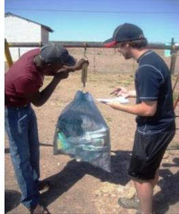
Figure 10. (Right) Quantifying solid waste output from households
