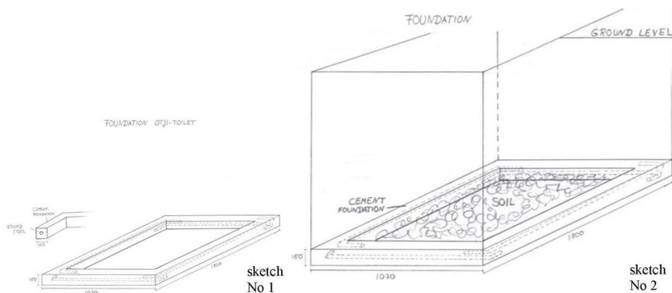
The concrete foundation will be reinforced with the round steel you received together with the Otji-Toilet self builder set. This reinforced foundation has to carry the whole weight of the toilet house and will prevent the walls from cracks. It is important to level the foundation exactly to get a straight toilet house. As a preparation for the concrete foundation dig a square channel of 150 mm depth and 150 mm wide on the ground of the hole.
