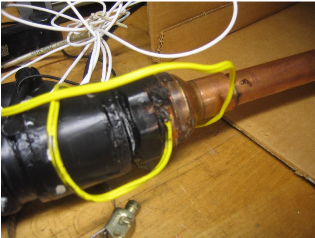
Figure 19 Shows thermocouples attached to the Cold Heat Exchanger side
