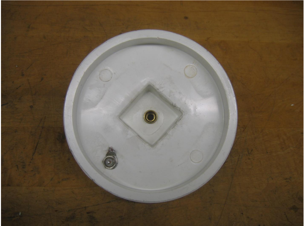
Figure 7 the bottom of the drain cap lid.
