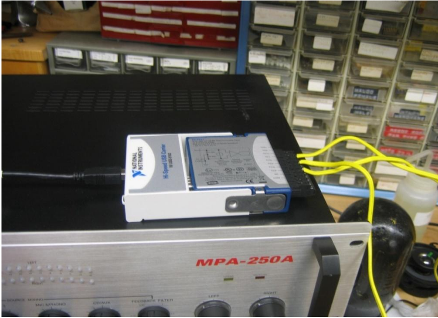
Figure 18 Type K thermocouples along with a NI hardware was used to measure temperature across the stack.
