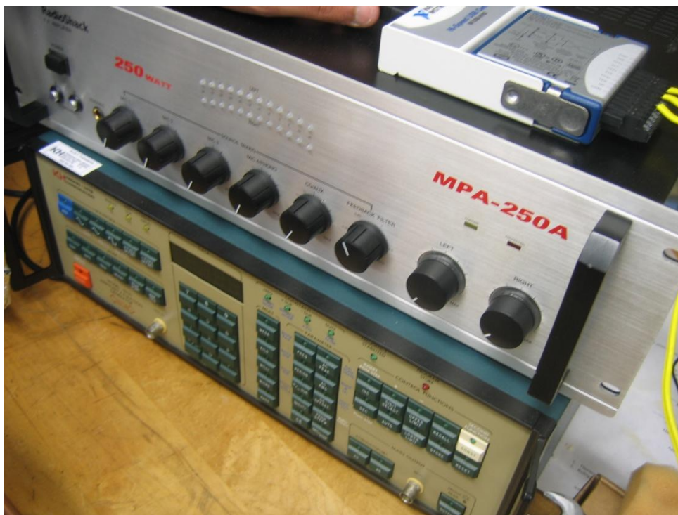
Figure 22 Shows the Radioshack Amplifier stacked on top of the Kronhite Wave Generator
