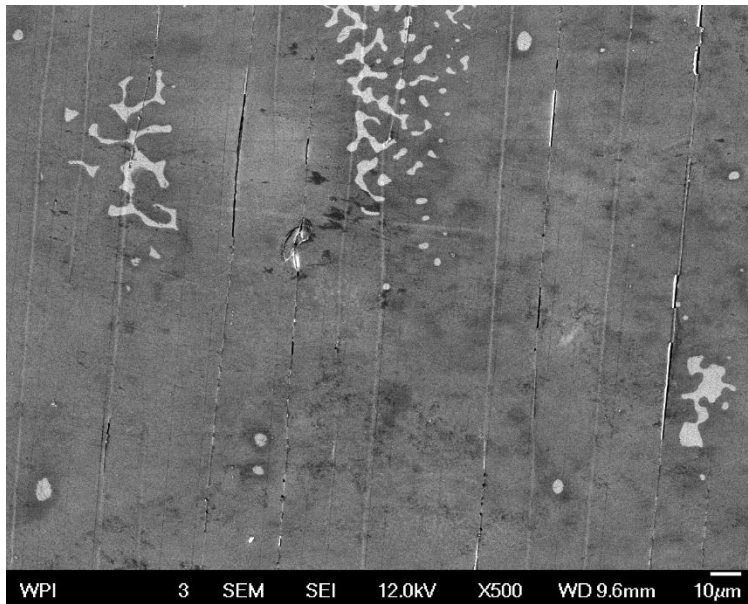
Figure 14 ITO Cracking after Bending 100 Times
