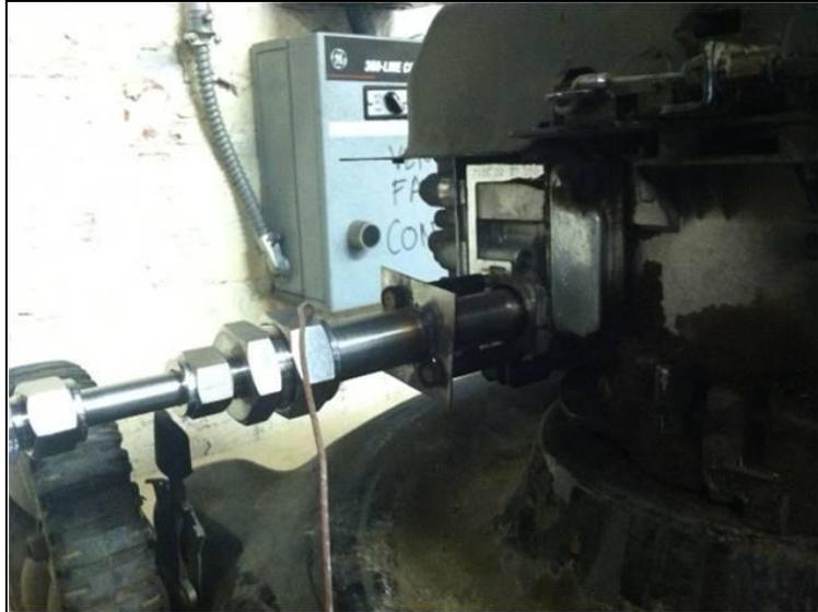
Figure 48: Exhaust outlet connecting to cooler
