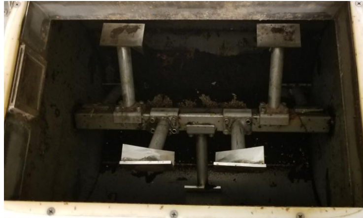
Figure i: interior view of the Worcester State University food dehydrator, displaying its pulping mechanism [Personal photograph taken at WSU]. (2019, March 29).
