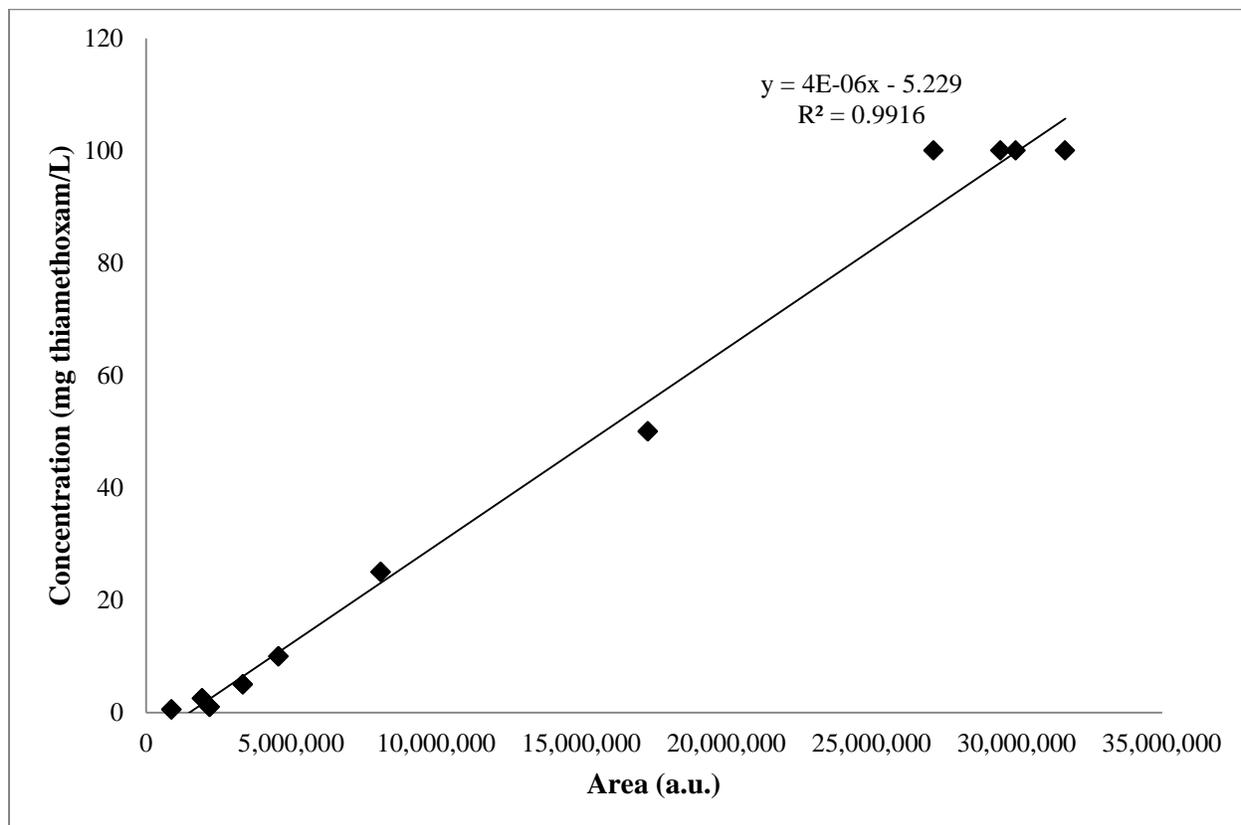
**Figure 8: Combined Calibration Curve for Correlating HPLC Absorbance to Concentration**
