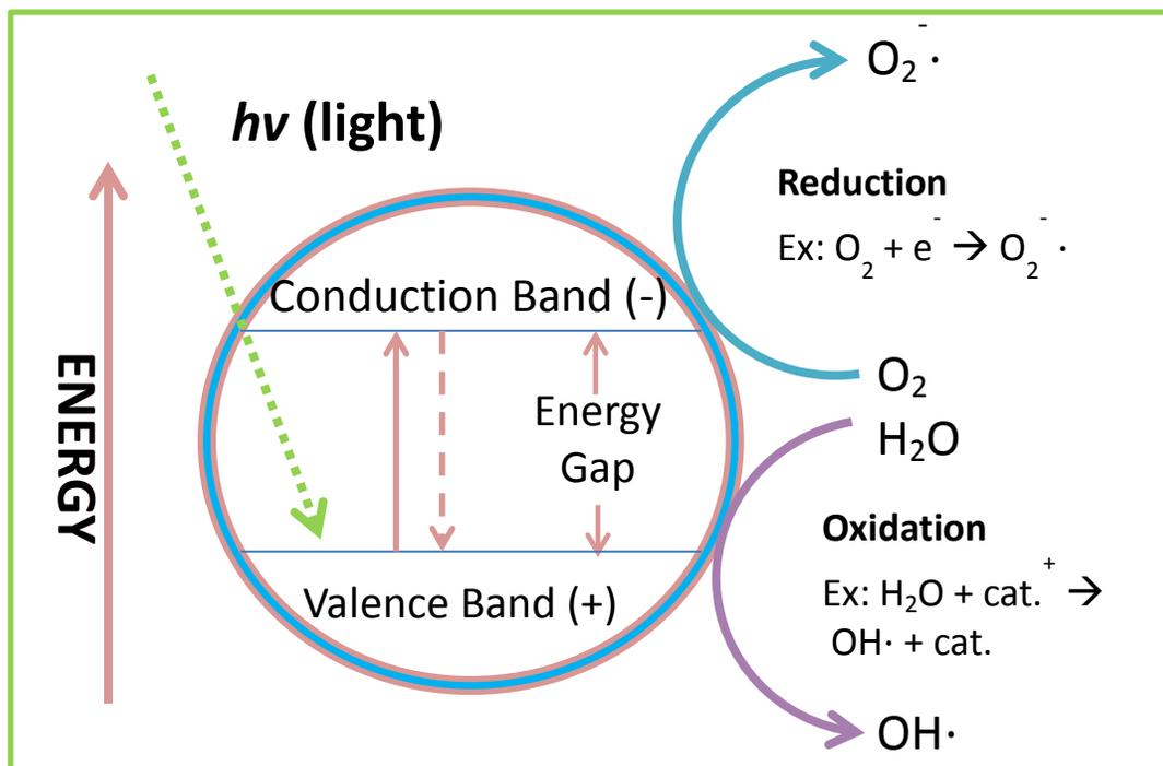
Figure 2: Photocatalysis Reaction Diagram, adapted from Photocatalysis (2005)
