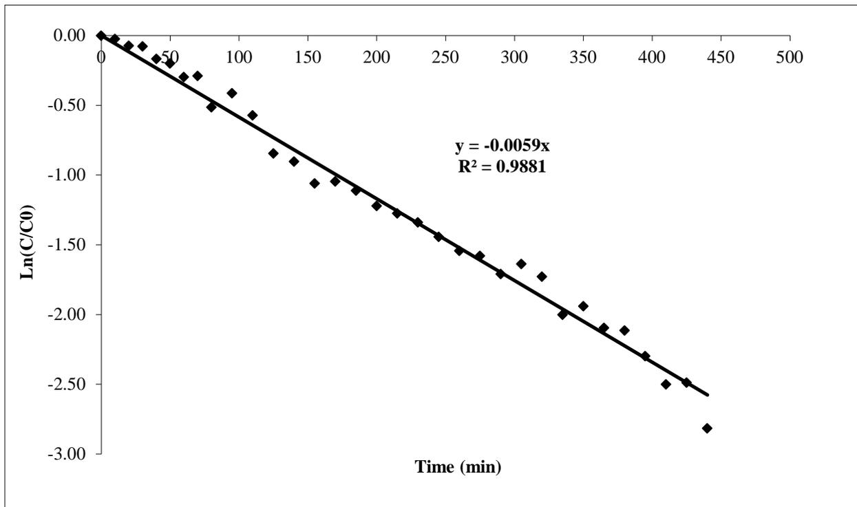
Figure 19: Kinetic Data for 30 ppm Thiamethoxam + 10 mg/L Humic Acid, Run 2
