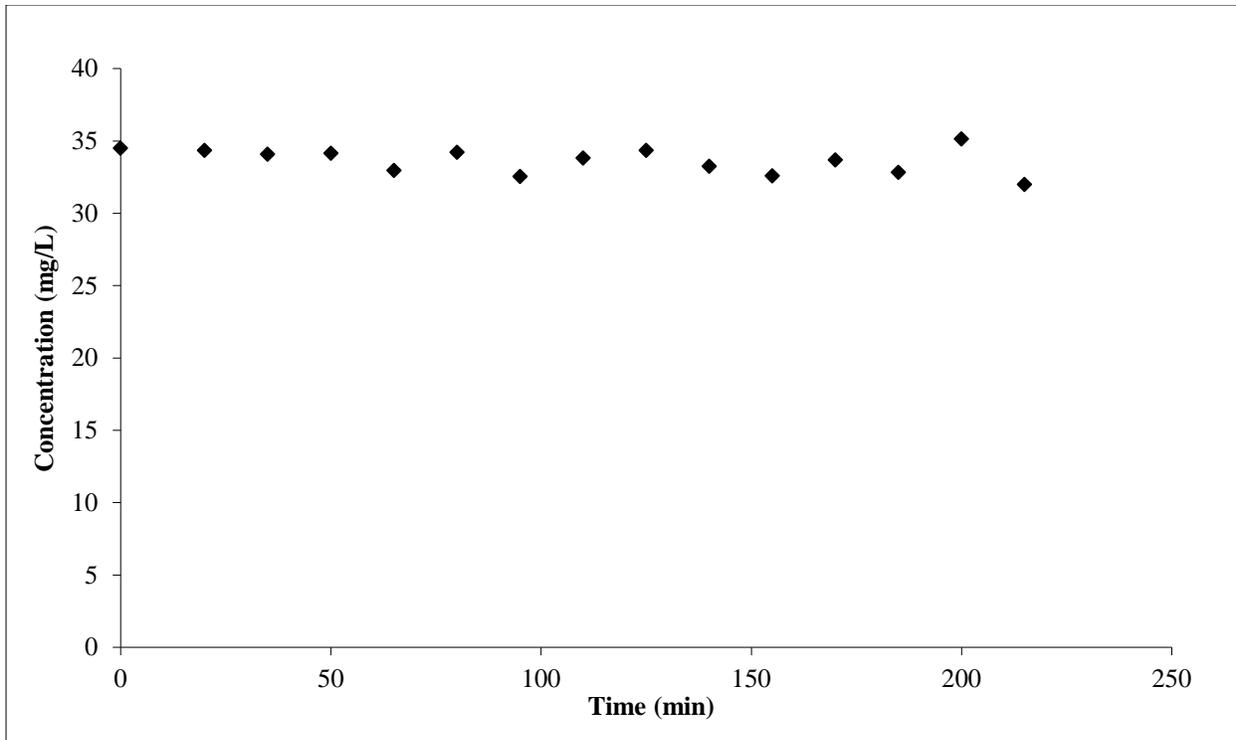
**Figure 10: Concentration Data for Thiamethoxam Experiment without UV light and with TiO<sub>2</sub>**
