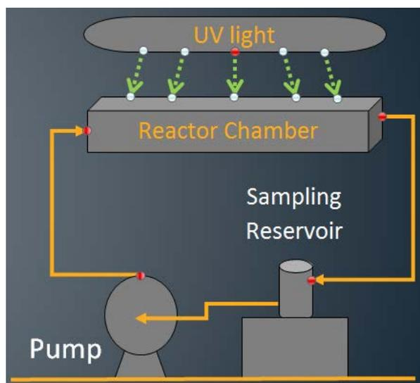
Figure 3: Schematic of Reactor System
