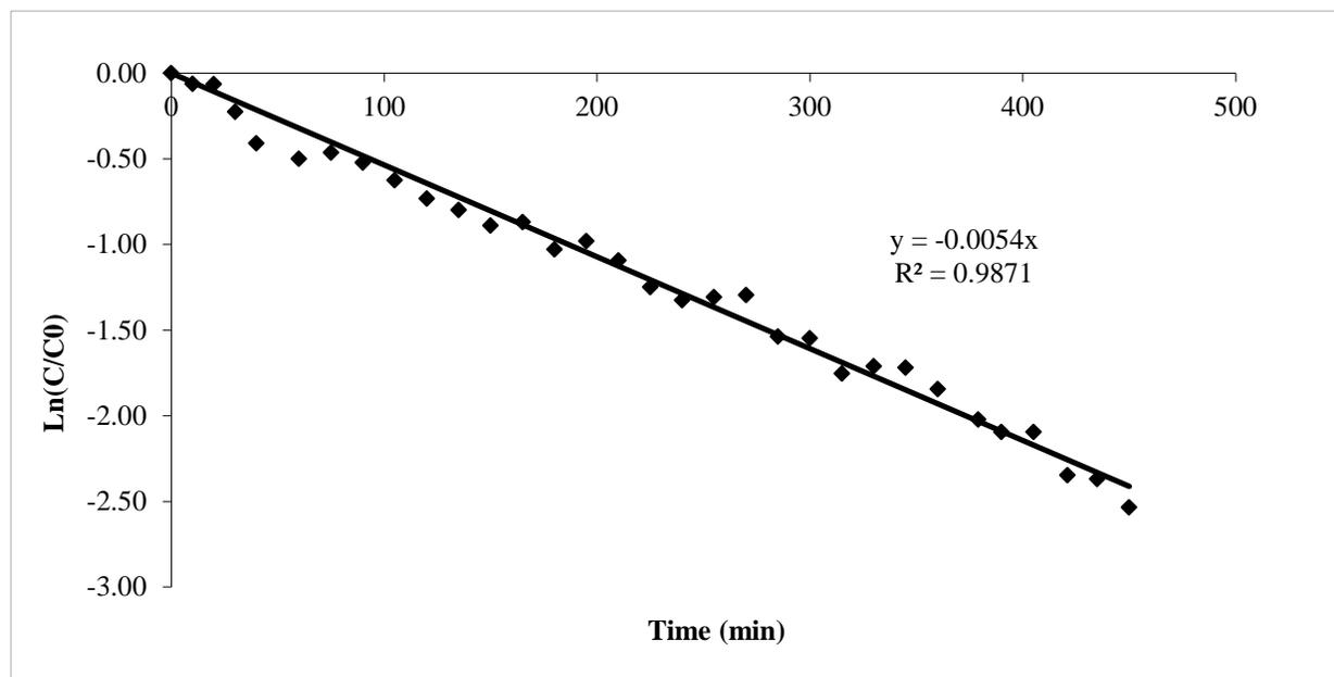
**Figure 5: 1st Order Rate Coefficient Graph for the Photocatalytic Degradation of 30 ppm Thiamethoxam**
