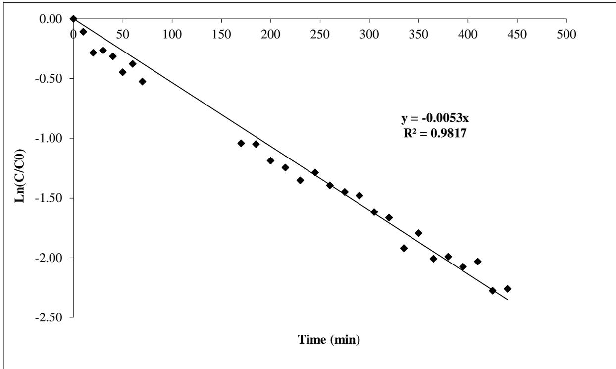
Figure 17: Kinetic Data for 30 ppm Thiamethoxam + 20 mg/L NH<sub>4</sub>NO<sub>3</sub>, Run 2
