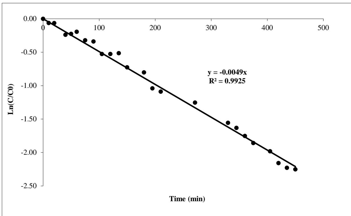
Figure 21: Kinetic Data for 30 ppm Thiamethoxam + 10 mg/L Humic Acid, Run 4
