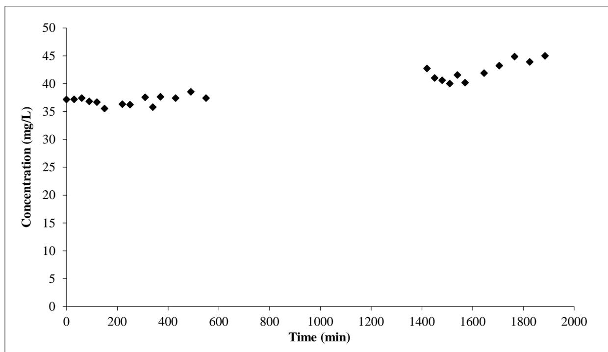
Figure 9: Concentration Data for Thiamethoxam Experiment with UV light and without TiO<sub>2</sub>
