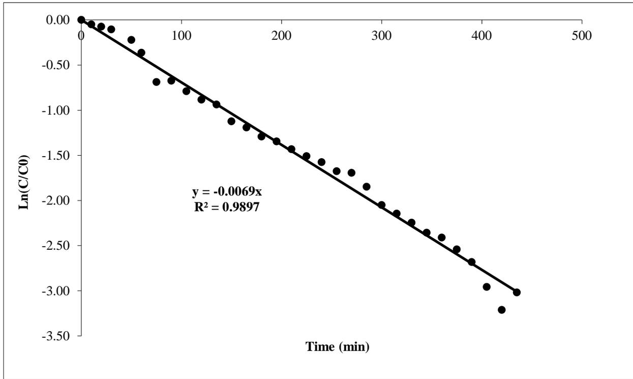
Figure 18: Kinetic Data for 30 ppm Thiamethoxam + 10 mg/L Humic Acid, Run 1
