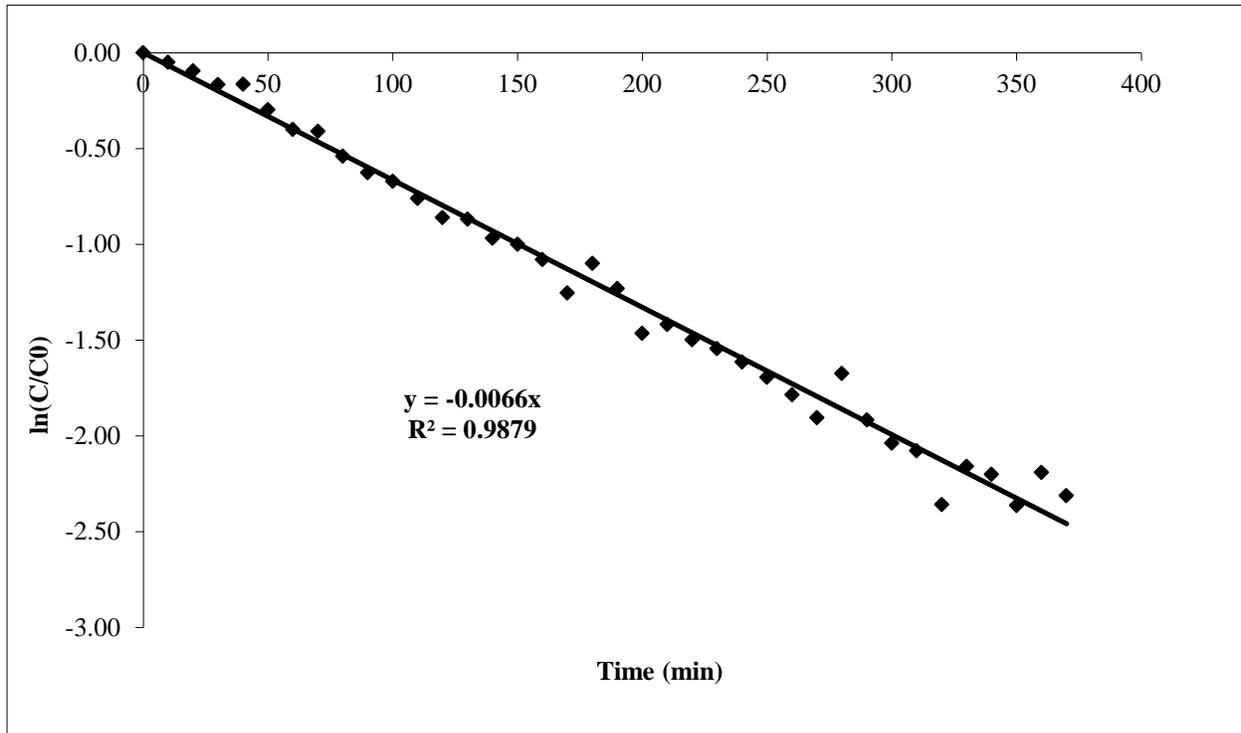
Figure 14: Kinetic Data for 30 ppm Thiamethoxam + 500 mg/L NH<sub>4</sub>NO<sub>3</sub>, Run 1
