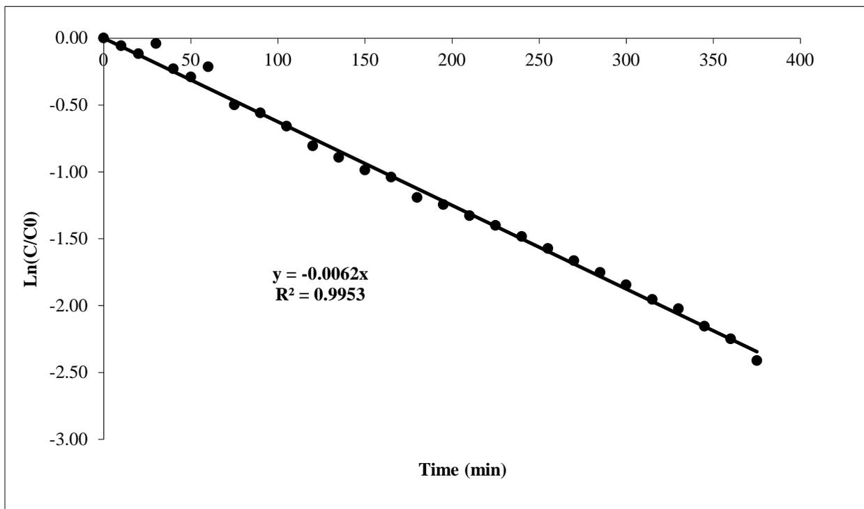
Figure 23: Kinetic Data for 30 ppm Thiamethoxam + River Water, Run 1
