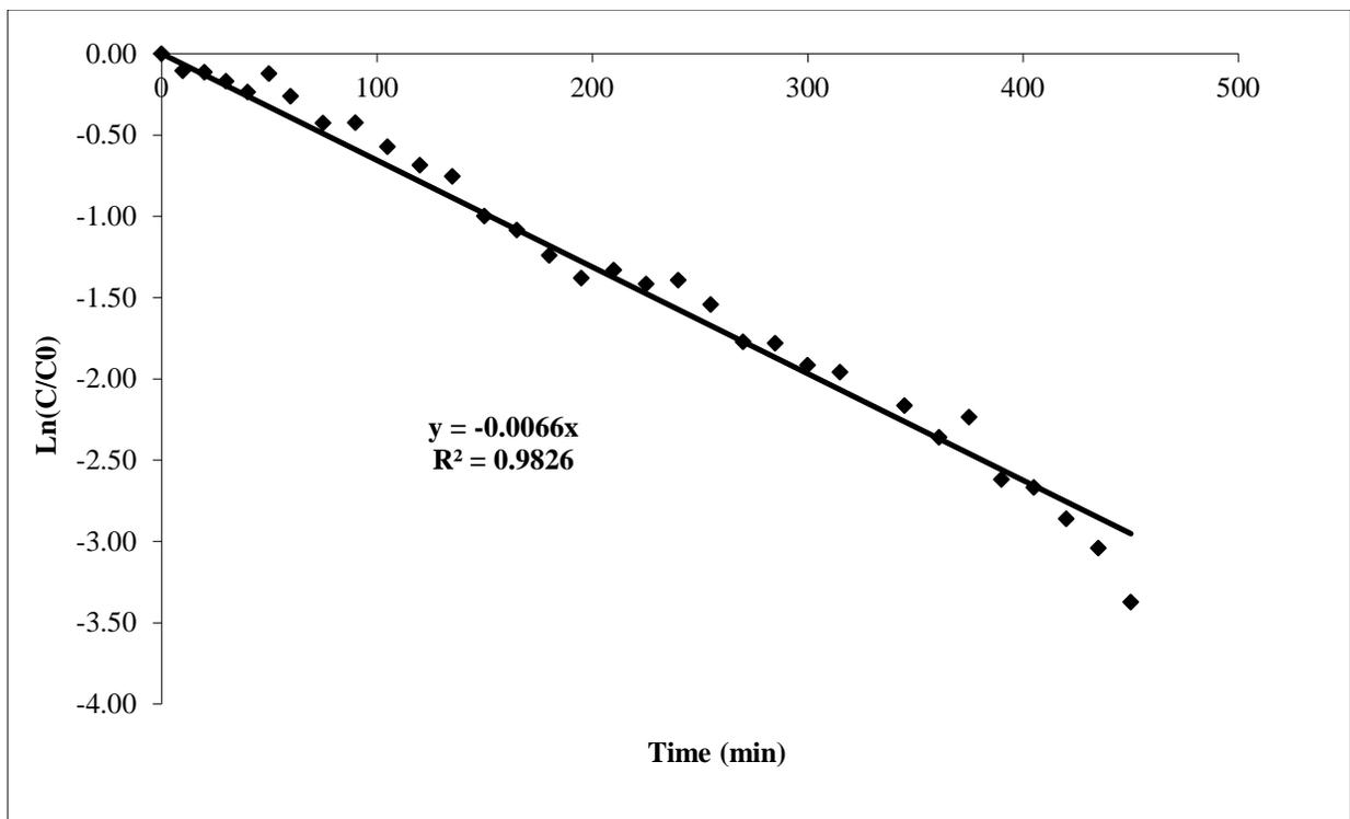
Figure 20: Kinetic Data for 30 ppm Thiamethoxam + 10 mg/L Humic Acid, Run 3
