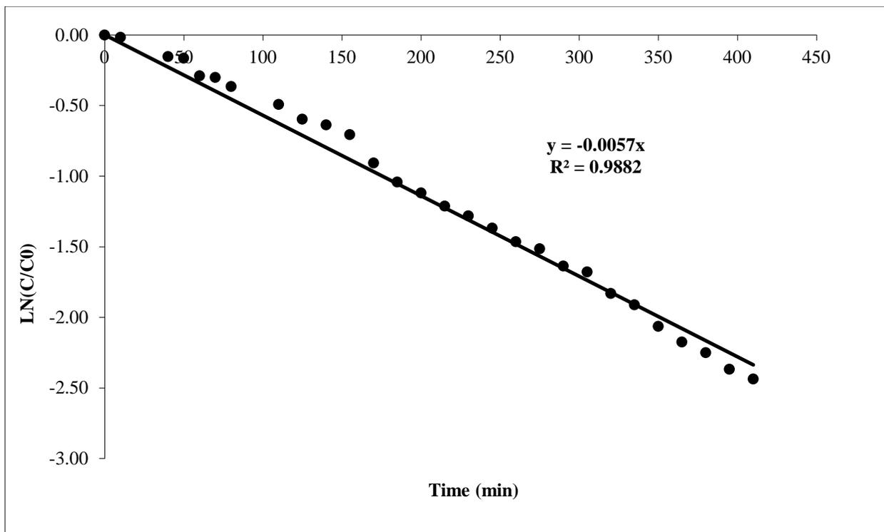
Figure 22: Kinetic Data for 30 ppm Thiamethoxam + 10 mg/L Humic Acid, Filtered
