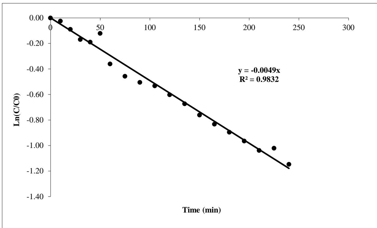
Figure 25: Kinetic Data for 30 ppm Thiamethoxam + River Water, Run 4
