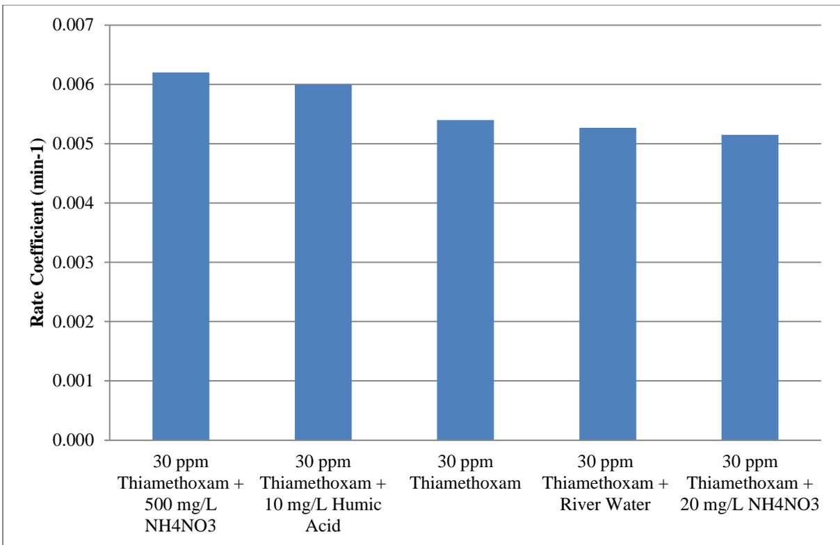
**Figure 6: Average Reaction Rate Coefficients**
