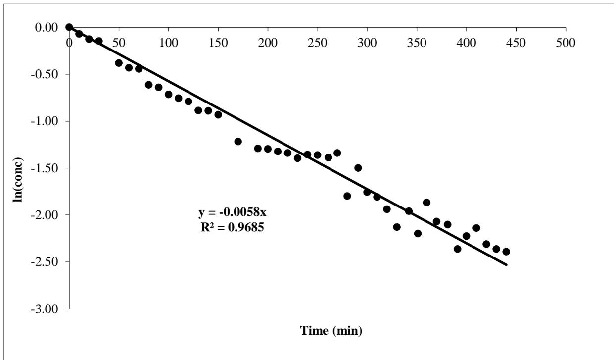
Figure 15: Kinetic Data for 30 ppm Thiamethoxam + 500 mg/L NH<sub>4</sub>NO<sub>3</sub>, Run 2
