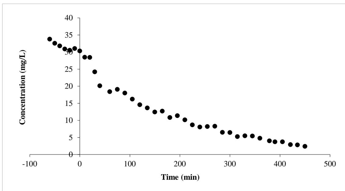
Figure 4: Concentration of 30 ppm Thiamethoxam vs. Time during Photocatalysis
