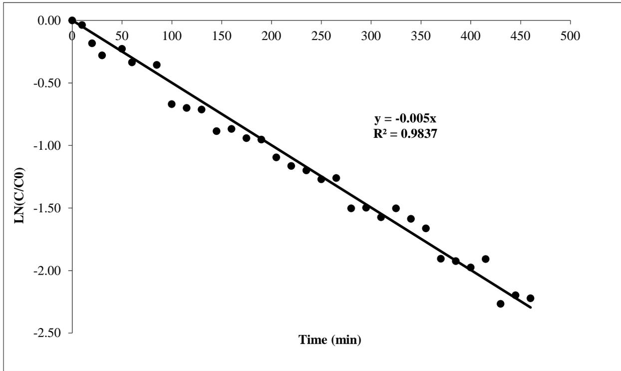
Figure 16: Kinetic Data for 30 ppm Thiamethoxam + 20 mg/L NH<sub>4</sub>NO<sub>3</sub>, Run 1
