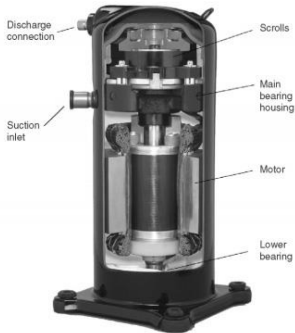
Figure 4.25 Cut away view of scroll compressor (Emerson Climate Technologies)
