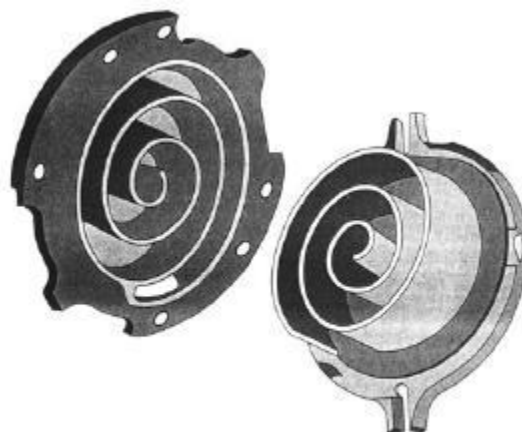
Figure 9-82 Two halves of the scroll compressor. (Courtesy of Lennox.)
