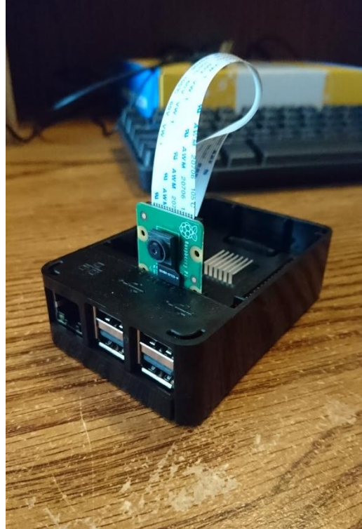
Figure 6: Raspberry Pi Camera Module and Motherboard Setup
