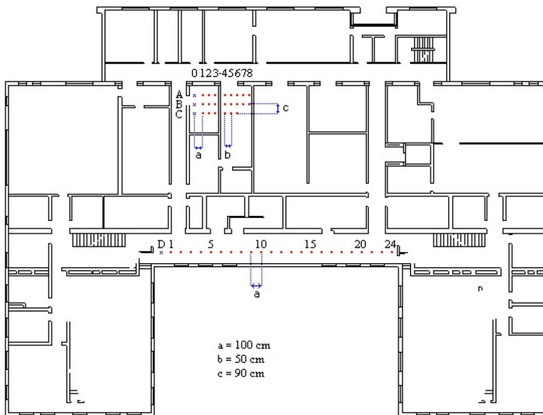
Figure 4.4: Measurement plan at 2 nd Floor with Tx located at A0, B0, C0, and D0, AK Laboratories
