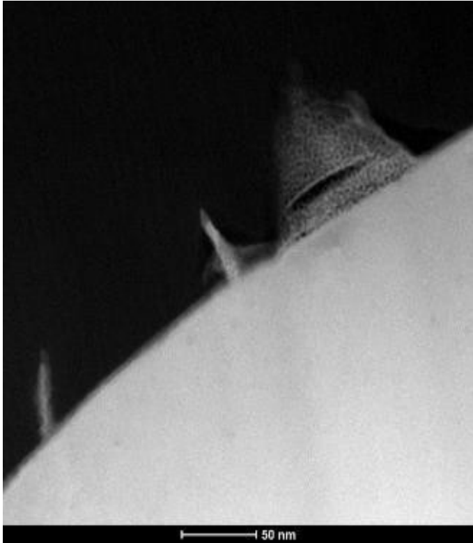
Figure 48. TEM of RH50% showing spikes protruding from the surface layer.
