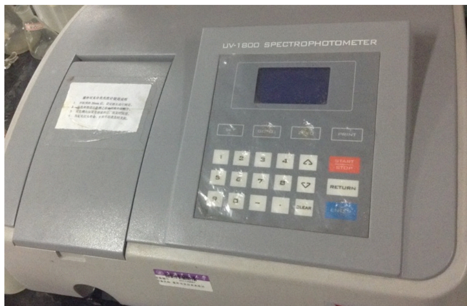
Figure 8 The spectrometer used for detecting HA concentration
