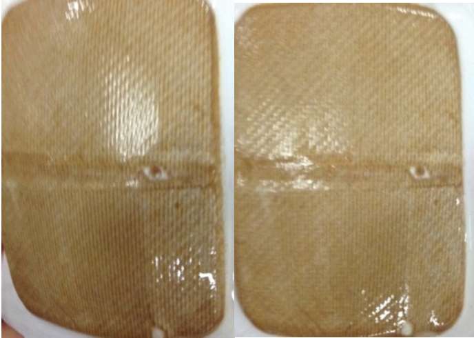
Figure 17 HA on the membrane, before and after cleaning with pure water
