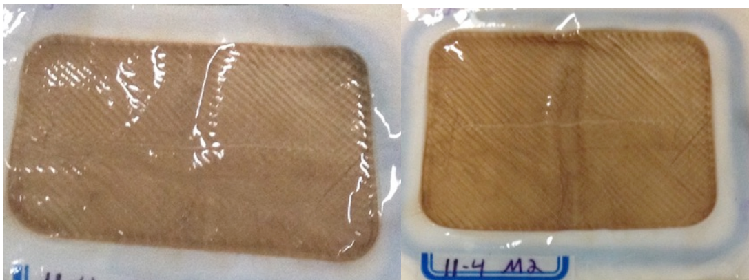
Figure 25 Before and after appearance of membrane cleaned with H 2 O 2
