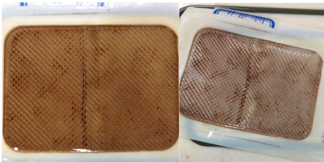
Figure 53 Post mechanical cleaning, then UV/H 2 O 2 AOP cleaning
