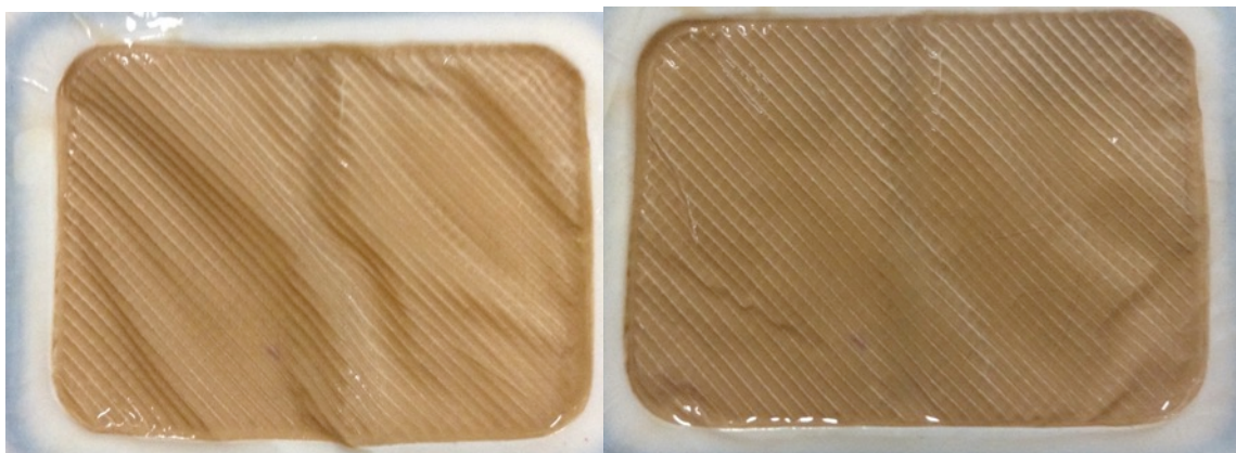
Figure 34 Before and after appearance of membrane cleaned with ozone/H 2 O 2
