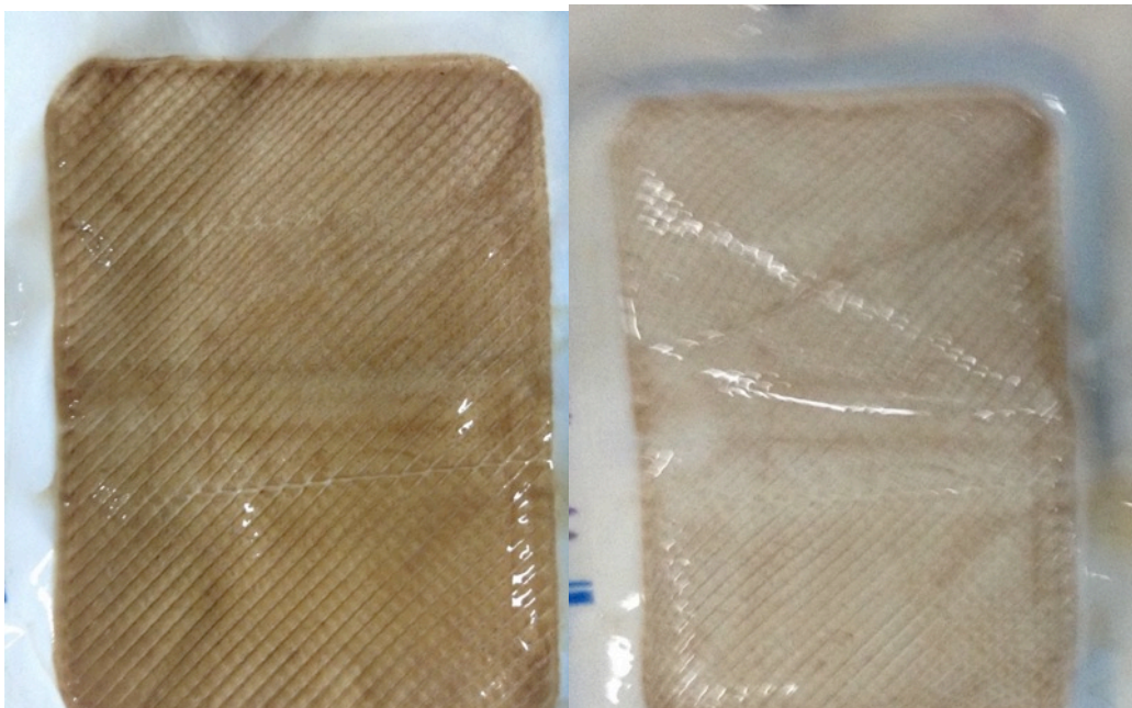
Figure 31 Before and after appearance of the membrane cleaning with UV/H 2 O 2
