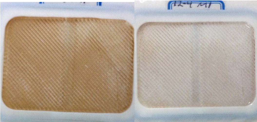
Figure 40 Before and after appearance of membrane cleaned with all AOPs
