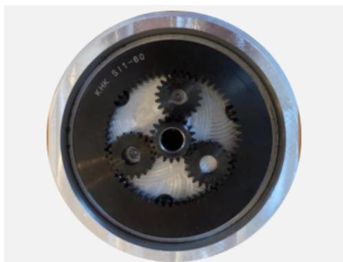
Figure 38: Planetary Gear system Parts within Female hinge
