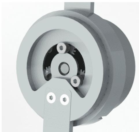
Figure 32: Moat Cut in the Assembly
