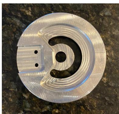
Figure 10: Manufactured Male Hinge
