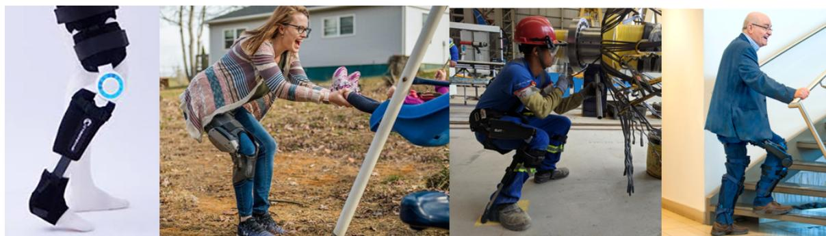
Figure 1: The existing devices from left to right: Cyberdyne's HAL Single Joint, Ottobock's C-Brace, SuitX's Leg X, B-Temia's KEEOGO. These images are adapted from, (Cyberdyne, n.d.), (Alex Hernandez, 2018), (SuitX, n.d.), (Keeogo, 2015)
