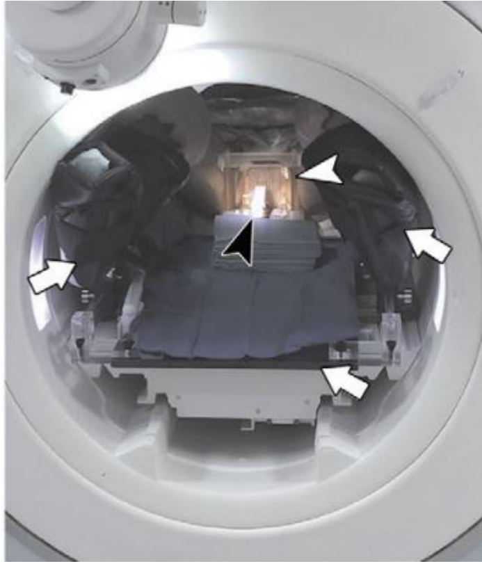
Figure 1.5: An in-bore view during manual insertion MRI-guided targeted biopsy. The white arrows show the patient table and foot rests while the template guide is shown with the white arrowhead and the inserted needle with the black arrowhead [25]
