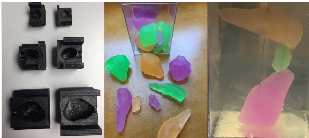
Figure 4.8: Molds of anatomical structures created from segmenting anonymized MR images. Left) The 3D printed molds, Center) structures molded from PVC, Right) a heterogeneous phantom assembled from the molds.
