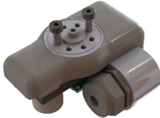
Figure 12: Close-up view of wrist joint, showing shoulder bolt interface
