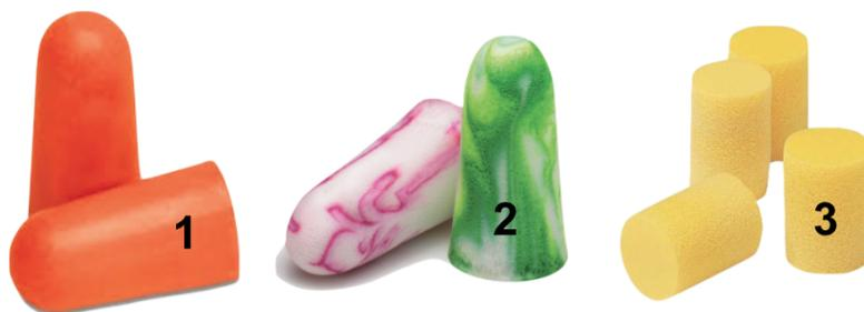
*Figure 37: Porous Earplug Samples Used for Testing. Chosen Because of Differing Material Properties, Pore Size, and Porosity*
