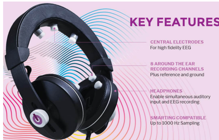
Figure 11. Diagram displaying the mBrainTrain Smartphones along with its three central electrodes, four other electrodes surrounding each ear, and some other device facts. (mBrainTrain, 2012)
