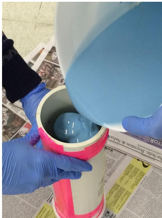
Figure 25 Creating tibia mold with Por-a-Mold
