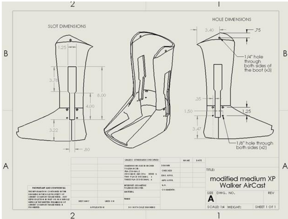
Figure 19 Medium XP Walker AirCast modifications
