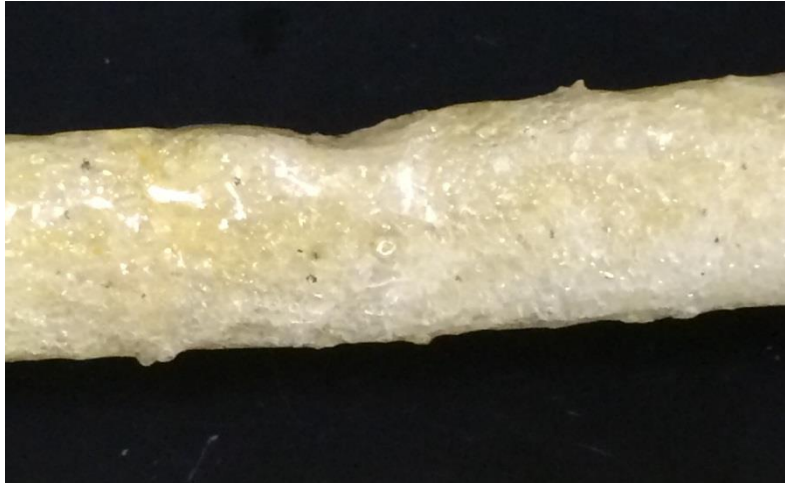
Figure 57 The deformation in the high-density polyurethane bone after testing
