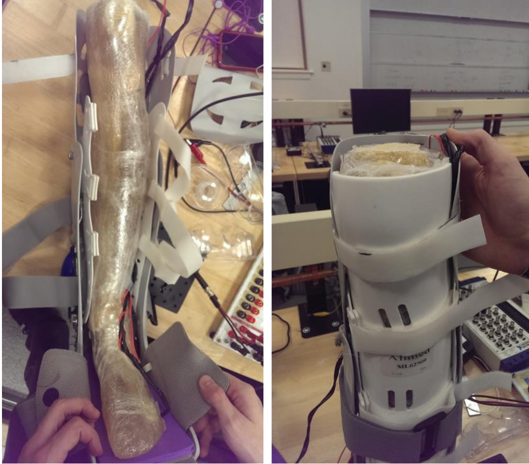
Figure 45 (a) Placement of leg model in the device over gap measurement padding and (b) a top view of the leg model inside the brace
