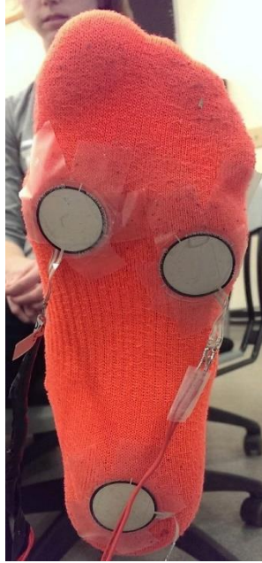
Figure 39 Force sensor locations on foot (bottom view)
