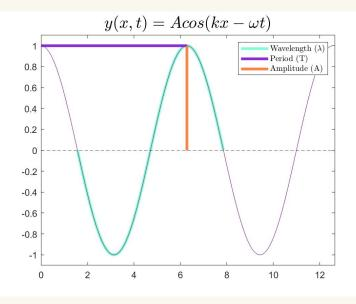
Sound is created by how a particle moves. The more distance the particle moves, the higher amplitude, the louder the sound is, while the smaller amplitude means a quieter sound. Another way for the sound to be varied is how long the wavelength is, the quicker the particle moves, the higher the pitch the sound is. The slower the particle moves, the lower the pitch of the sound. Think of this as how far the particle will move along its path in one second.
