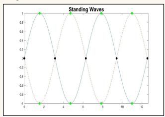
*Note.* For a standing wave in a string instrument, the x-axis is position, and the y-axis
