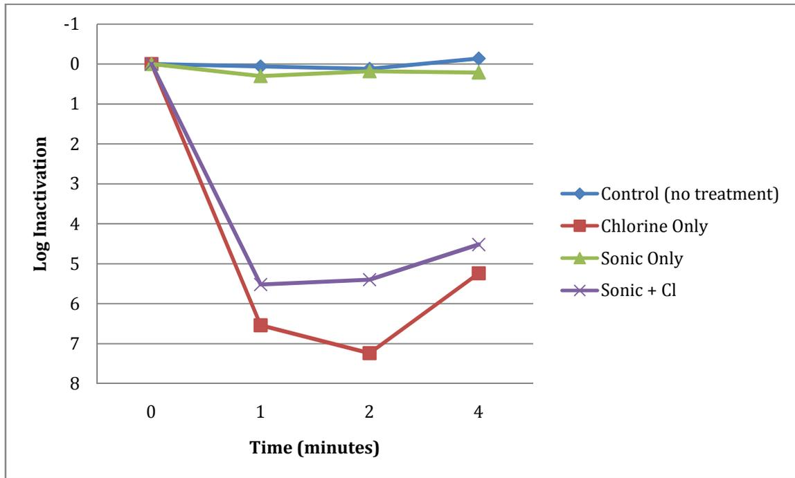
Figure 4-4: Log inactivation of *E. coli* with cavitation system (performed at WPI)
