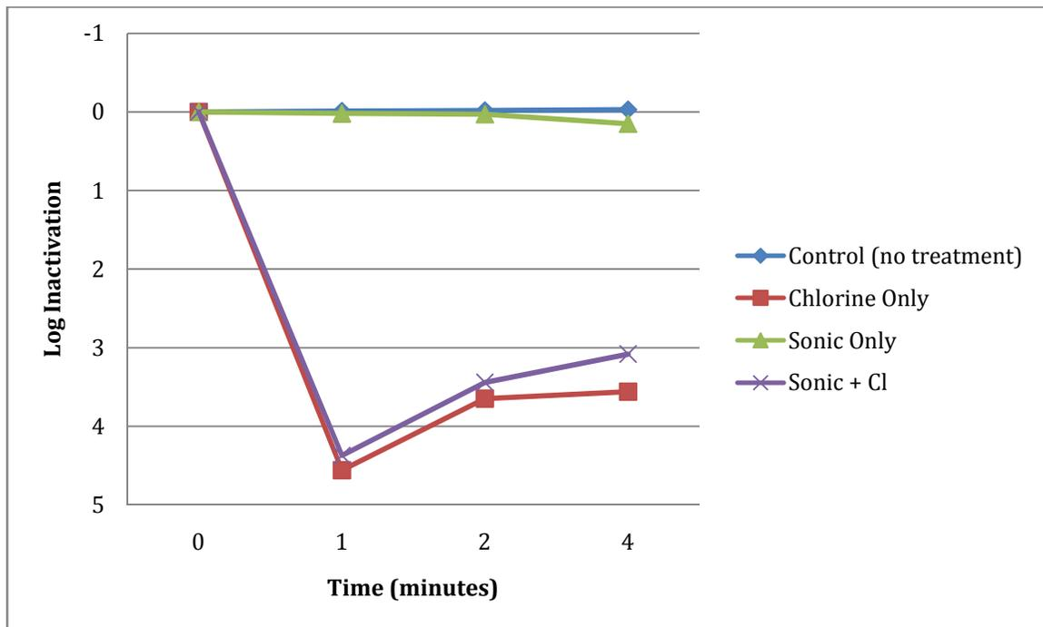
Figure 4-5: Log inactivation of *E. coli* with circulating cavitation system (performed at WPI)
