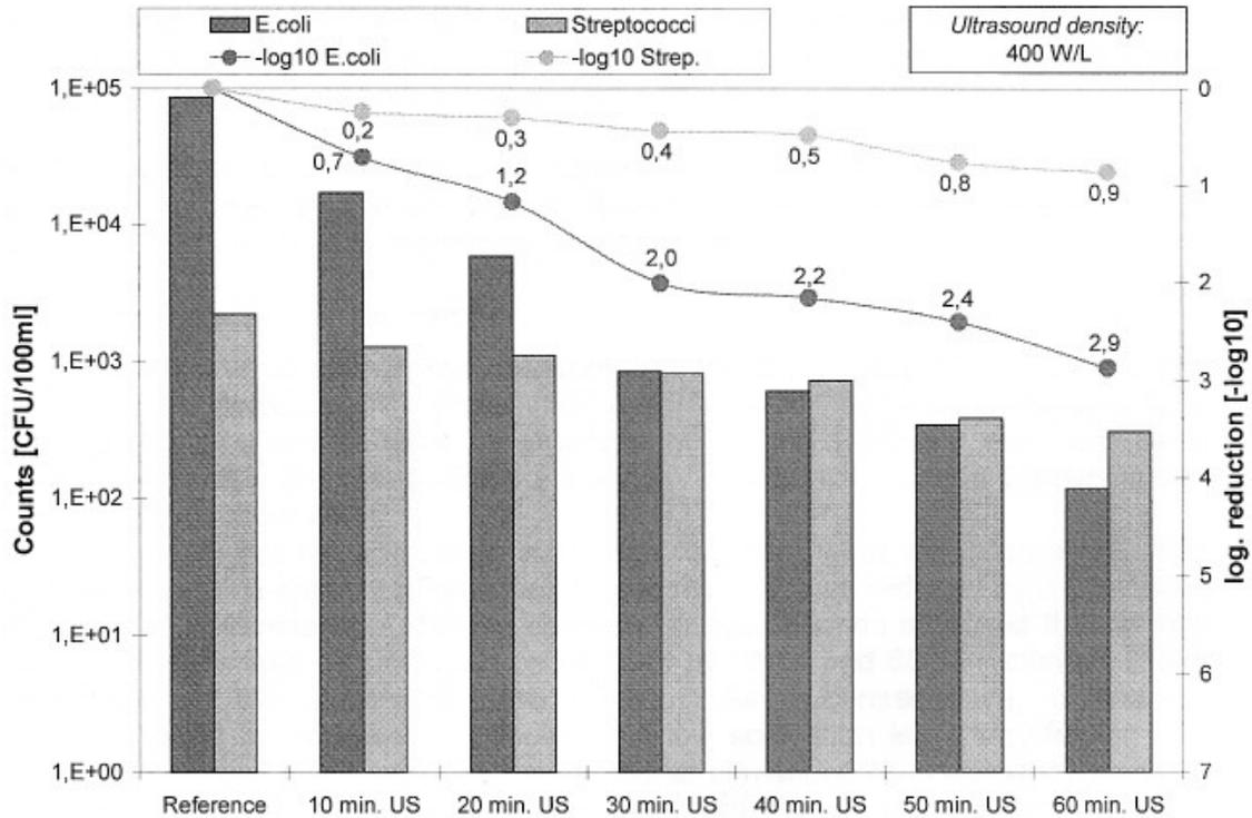
Figure 2-1: Inactivation on *E. coli* and fecal streptococci by sonication (Blume, Martinez and Uwe 2002)
