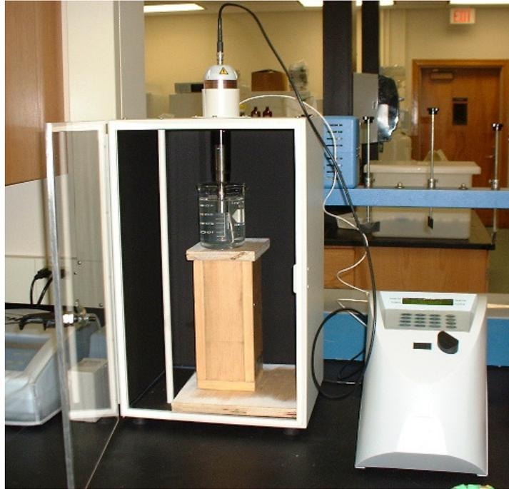
**Figure 3-1: Misonix probe sonication system**
