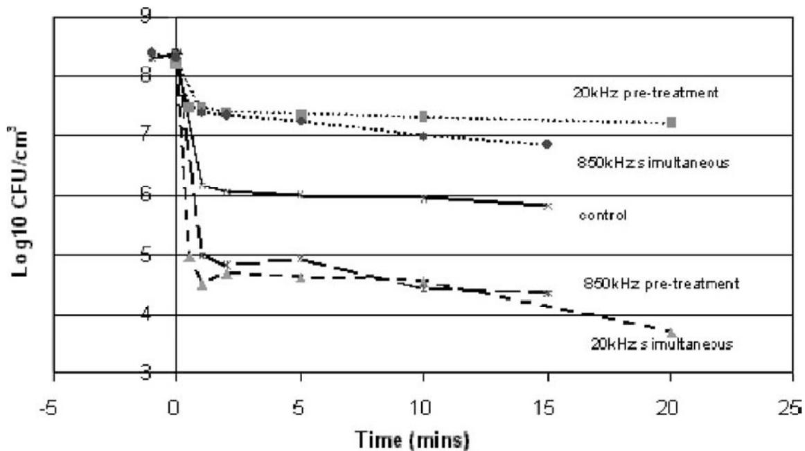
Figure 2-3: Chlorine inactivation of *E. coli* with pre- and simultaneous sonication for 1 minute (Duckhouse, et al. 2004)
