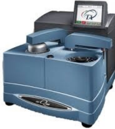
Figure 2.1. Modulated Differential Scanning Calorimetry model Q200 from TA Instruments, USA [9].
