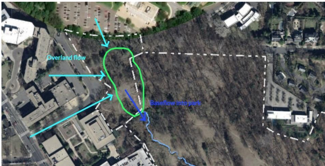
Figure 16: The LID (green outline) capturing all overland runoff and supplying base flow into the stream
