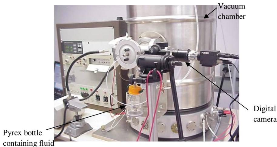
Figure 3.1 Facility used for electrospray including the vacuum chamber, Pyrex bottle containing fluid and digital camera to monitor the Taylor cone and jet.
