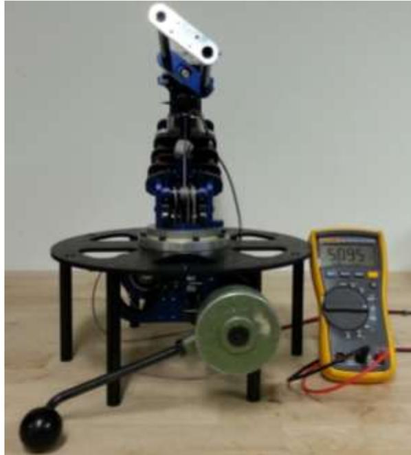
Figure 4-3: Torque Gauge Test
