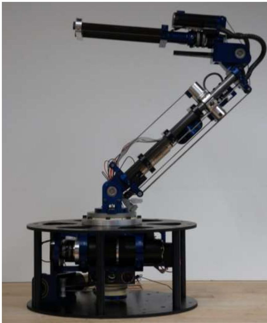
Figure 4-1: Assembled Arm
