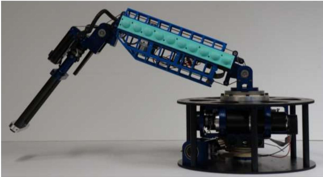
Figure 5-1: Complete First Four DOF of Robotic Arm
