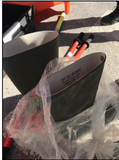
Figure 50: Rubber boots firefighters wear to withstand 20,000 volts of power when in a highly electric environment
