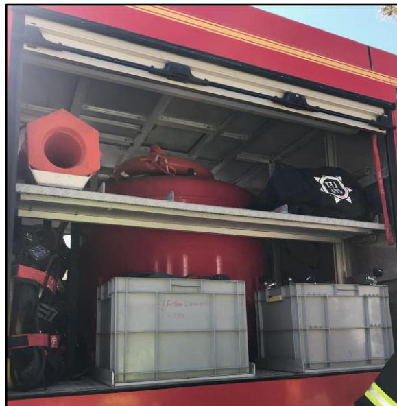
Figure 45: One ton foam tank located in the center of the OCP fire truck
