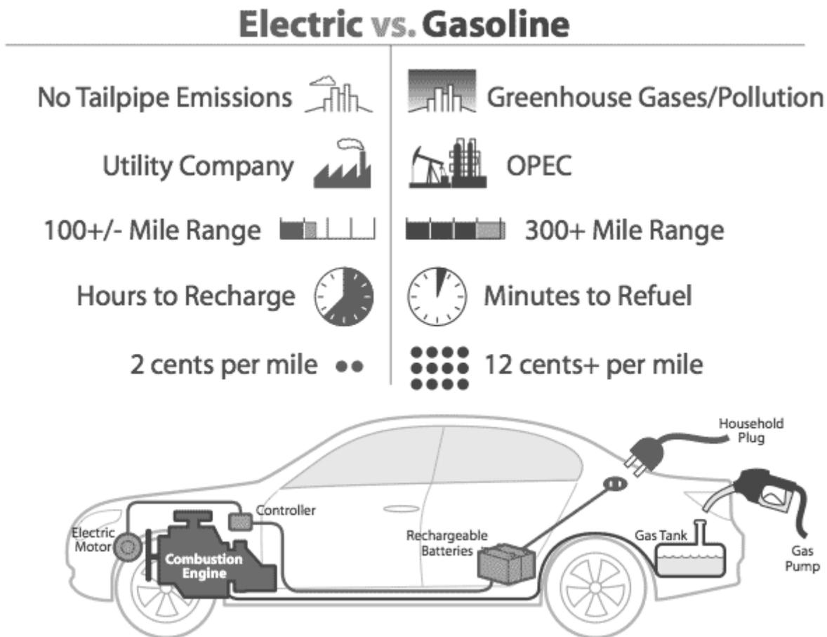
Figure 17: Electric vs. Gasoline<sup>45</sup>
