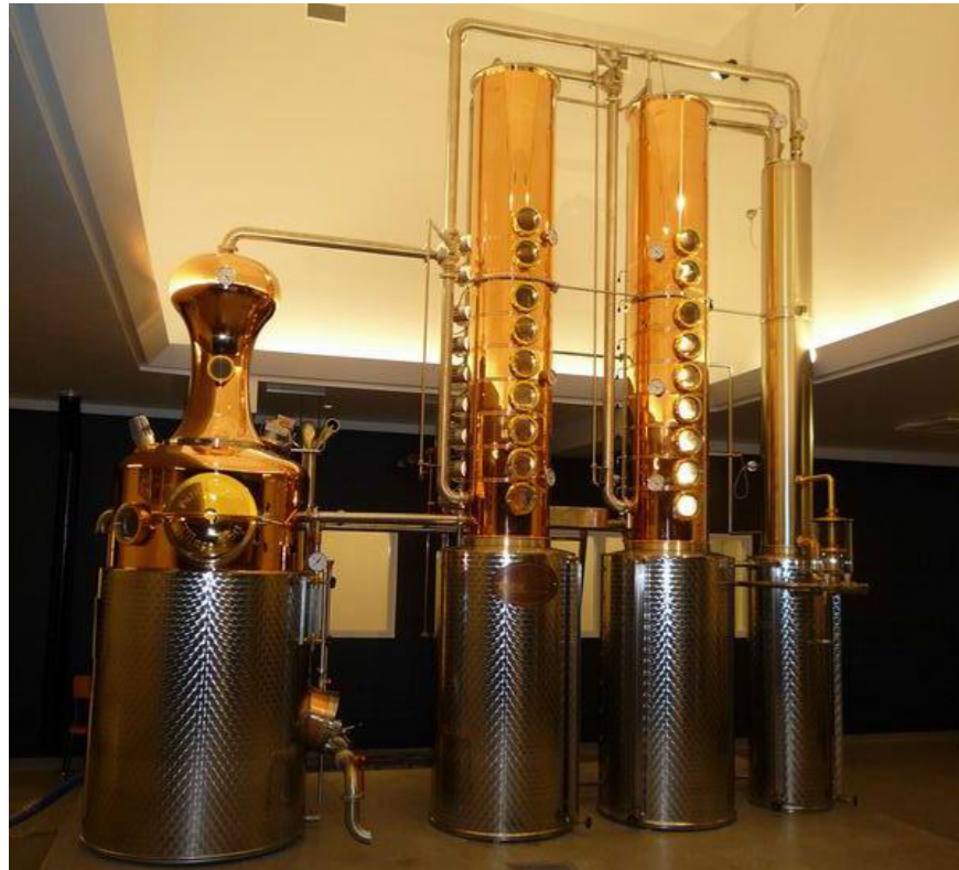
Figure 8: Kothe 600 L Twin Column Vodka Still
