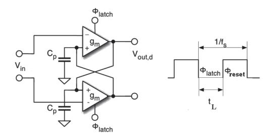
Figure 4.7: Regenerative latch structure [2]
