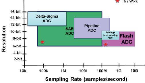
Figure 2.10: Different ADC architectures comparison [4]
