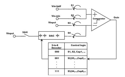
Figure 6.1: Proposed SA-ADC architecture
