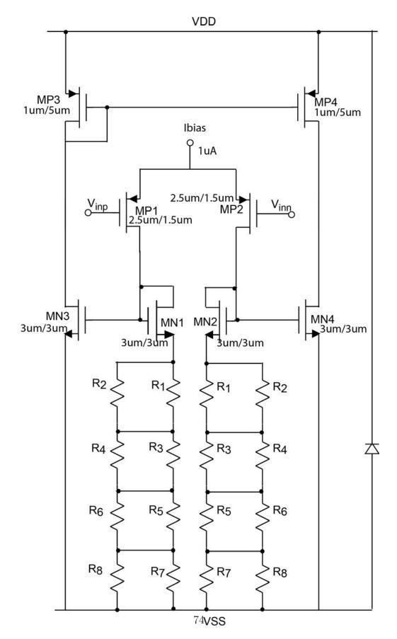
Figure 6.7: Analog buffer with tuning
