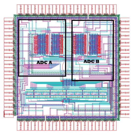
Figure 5.2: Flash ADCs Layout
