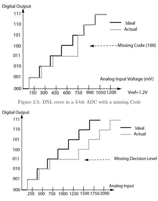
Figure 2.6: DNL error in a 3-bit ADC with missing Decision Levels
