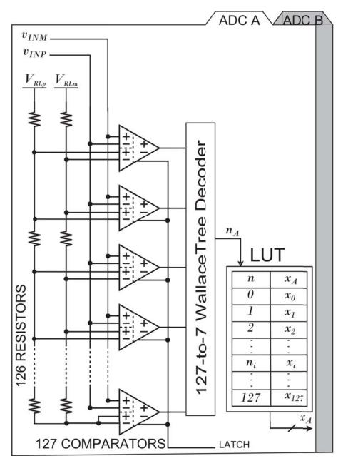
Figure 3.1: Block diagram of split redundant flash ADC
