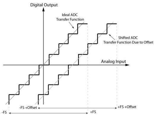
Figure 2.3: ADC Offset error
