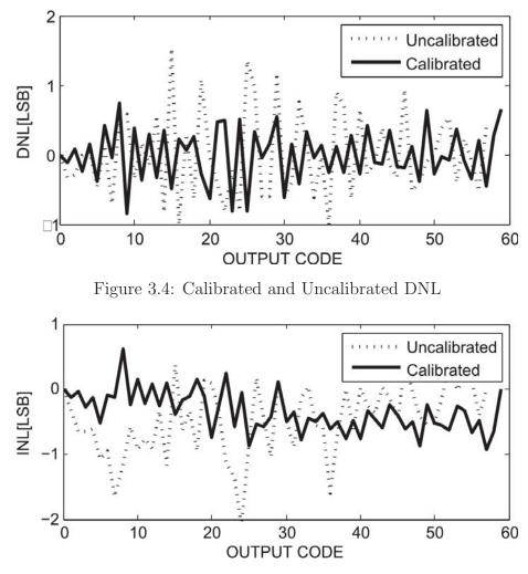
Figure 3.5: Calibrated and Uncalibrated INL
