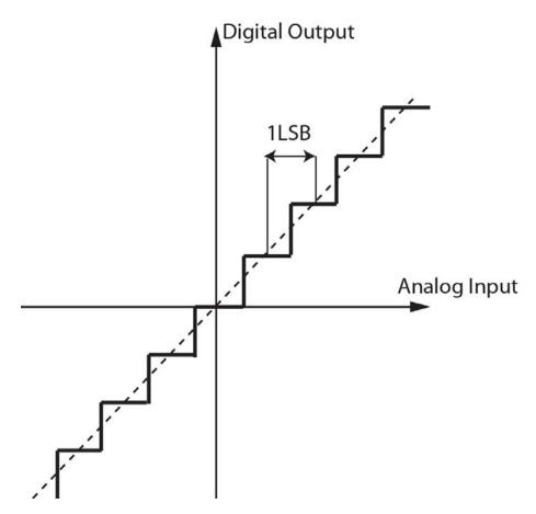
Figure 2.1: Ideal ADC transfer function
