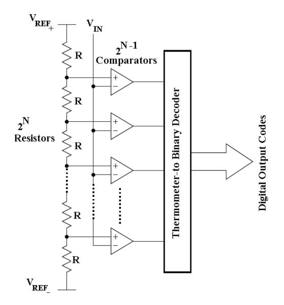
Figure 2.11: Block diagram of a flash ADC
