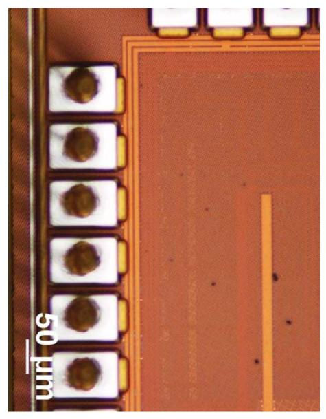
Figure 5.13: Closer view of ESD and bond pads
