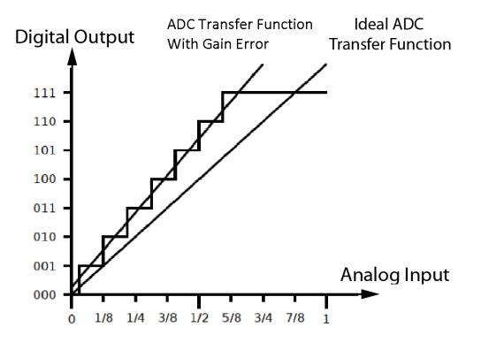
Figure 2.4: ADC Gain error
