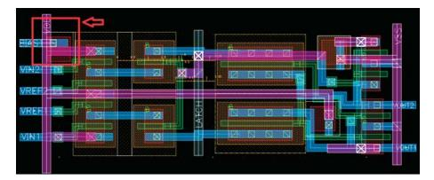
Figure 5.14: Layout mistake on PMOS substrate contact
