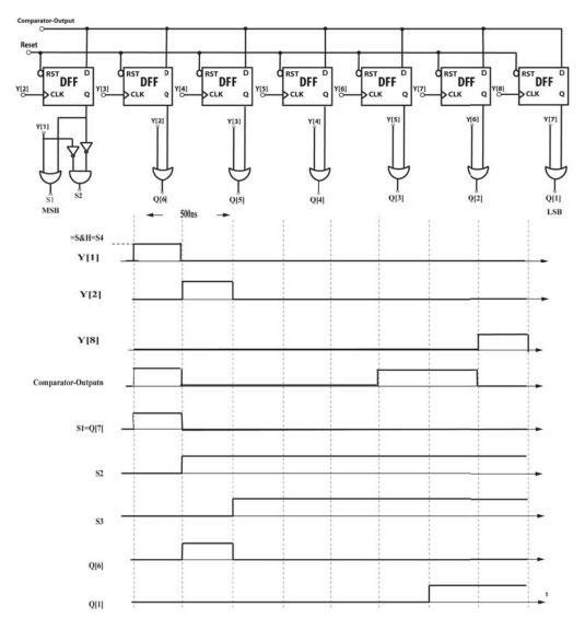
Figure 6.5: Control logic switches and timing
