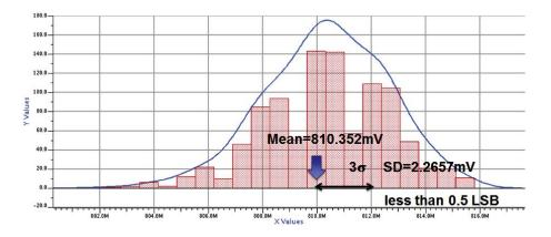
Figure 6.4: Monte-Carlo simulation of comparator offset.  $\sigma = 2.26 \text{mV}$
