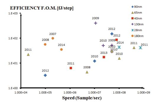
Figure 2.17: Survey of SAR ADCs.
