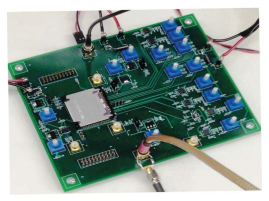
Figure 5.8: PCB board for flash ADC evaluation
