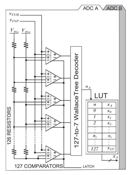
Figure 4.1: Block diagram of split redundant flash ADC
