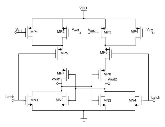
Figure 4.2: Block diagram of dynamic comparator
