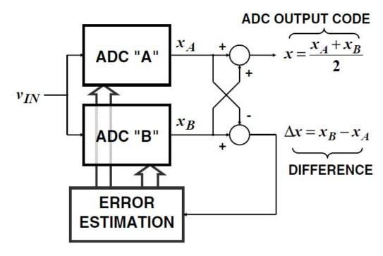
Figure 2.14: Split ADC Architecture [6]
