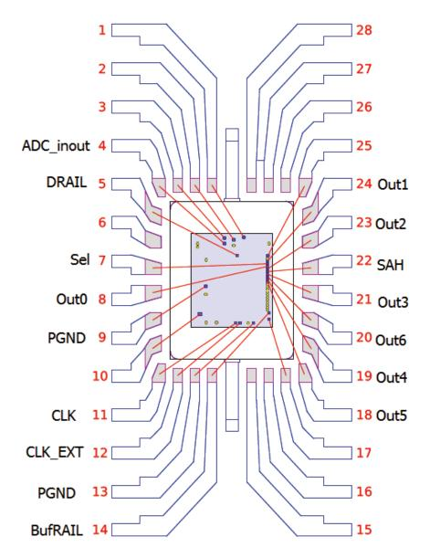
Figure 7.2: SAR ADC bonding diagram
