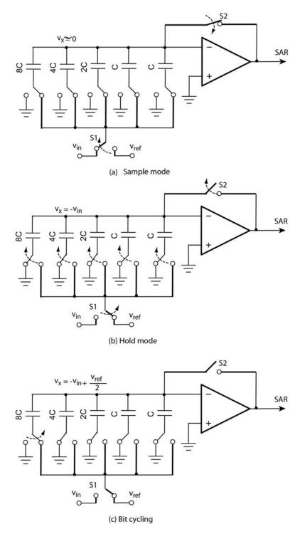
Figure 2.13: A 4-bit charge-redistribution SAR ADC [5]
