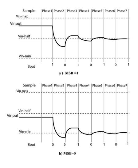
Figure 6.2: Waveforms of proposed switching procedure: (a) MSB=1 (b) MSB=0
