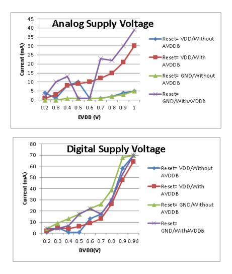
Figure 5.11: ESD test for flash ADC evaluation
