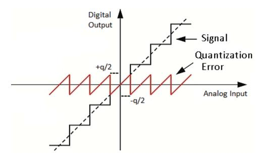
Figure 2.2: Quantization Error as a function of input voltage [1]
