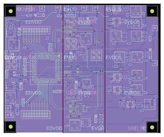
Figure 5.7: PCB layout for flash ADC evaluation
