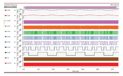
Figure 5.9: Simulation results for redundant flash ADC evaluation
