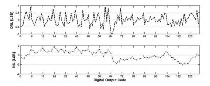
Figure 7.5: Measured DNL and INL with ramp input for Die2
