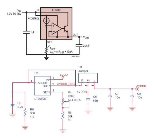
Figure 5.3: Linear regulators with low dropout voltage
