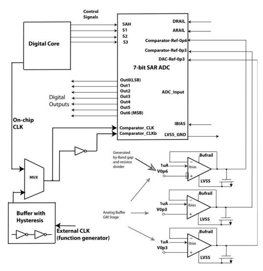
Figure 6.6: Top level schematic of SAR ADC design
