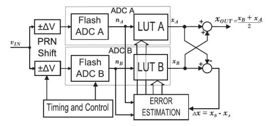
Figure 3.2: System block diagram
