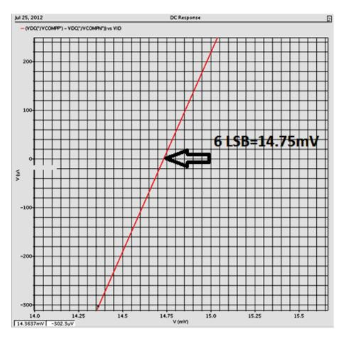
Figure 4.13: Analog shift simulation result: DC response
