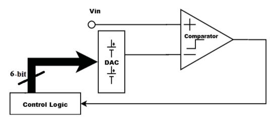
Figure 2.12: SAR ADC architecture
