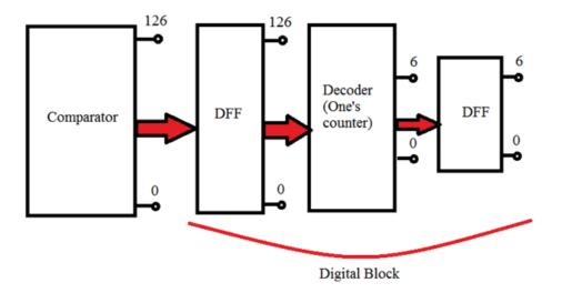
Figure 4.14: Digital block diagram of flash ADC
