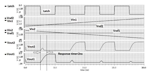
Figure 4.3: Dynamic comparator simulation results
