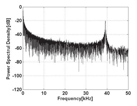
Figure 7.6: Measured 4096-point FFT spectrum at 100 kS/s.
