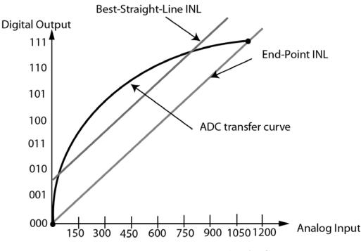
Figure 2.7: INL error in a 3-bit ADC
