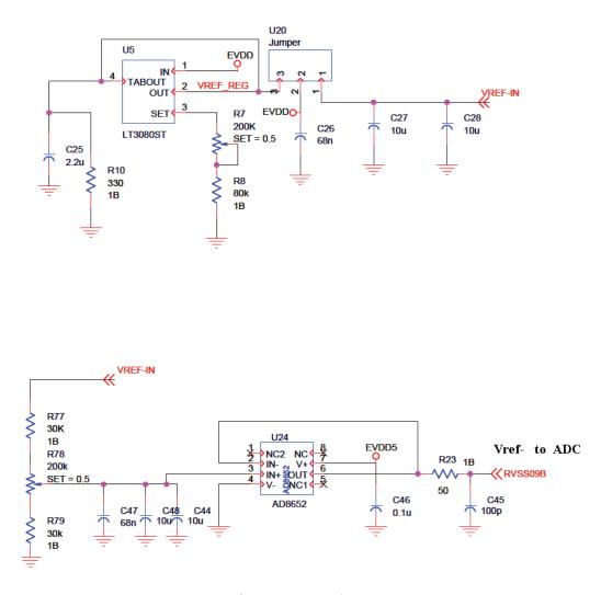
Figure 5.4: Generating reference voltages
