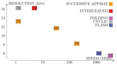
Figure 2.18: Survey of ADCs using "Split ADC" approach.
