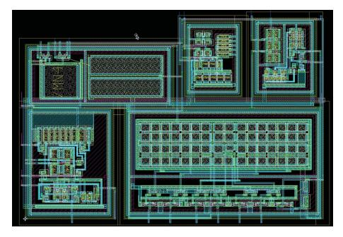
Figure 7.1: Analog portion of SAR ADC layout, including buffers, switches, DAC and comparator
