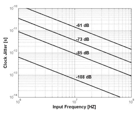
Figure 2.8: Sampling Jitter at different SNR and input frequency [2]
