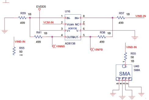
Figure 5.5: Generating differential input for each flash ADC
