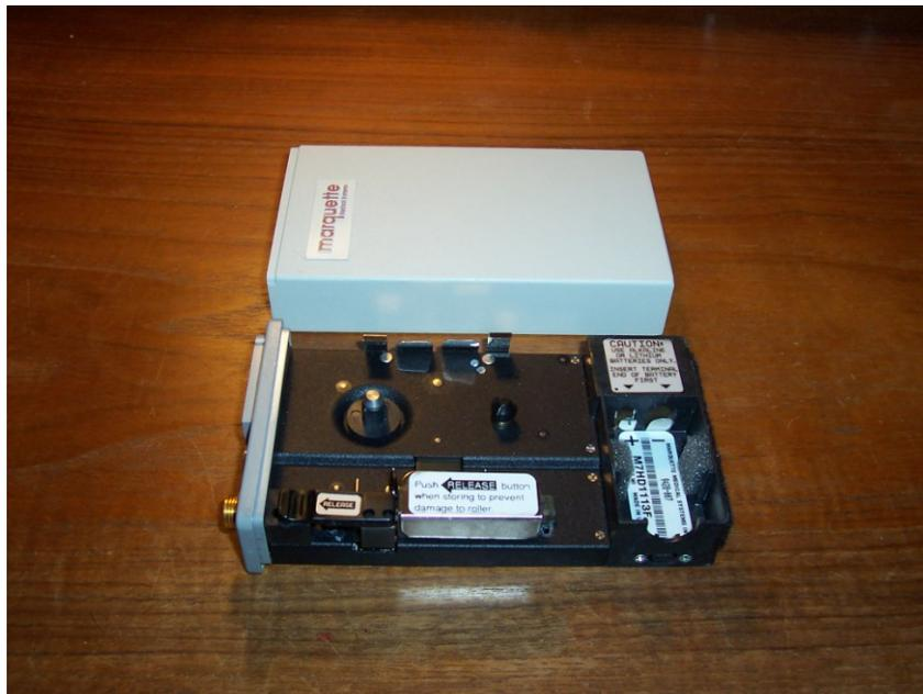
**Figure G.3: Internal view of Marquette holter monitor**
