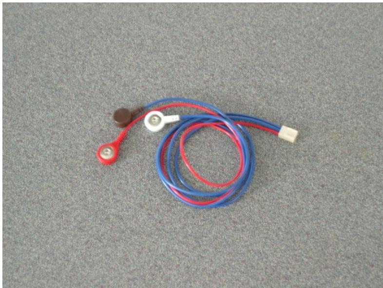
Figure 6.29: ECG electrode leads
