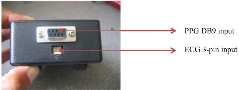
**Figure 6.35: Device hardware inputs**
