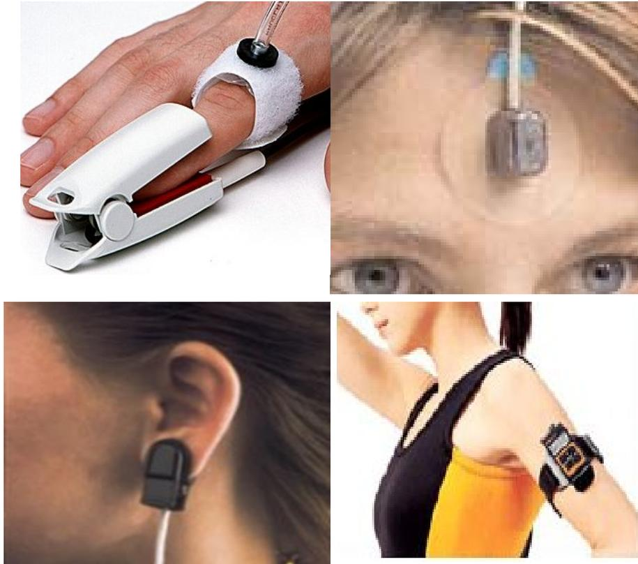
Figure 5.2: PPG Sensor location alternatives [28], [46]-[47]
