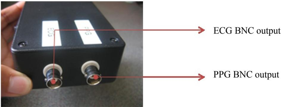
**Figure 6.36: Device hardware output connections**
