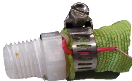
Figure 8: Muscle with wire running out of latex tube for measuring water resistivity
