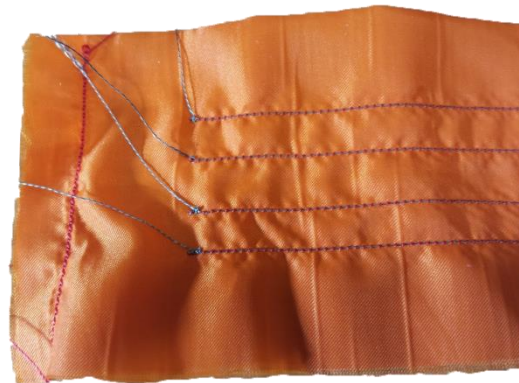
Figure 15: Parachute material with conductive thread
