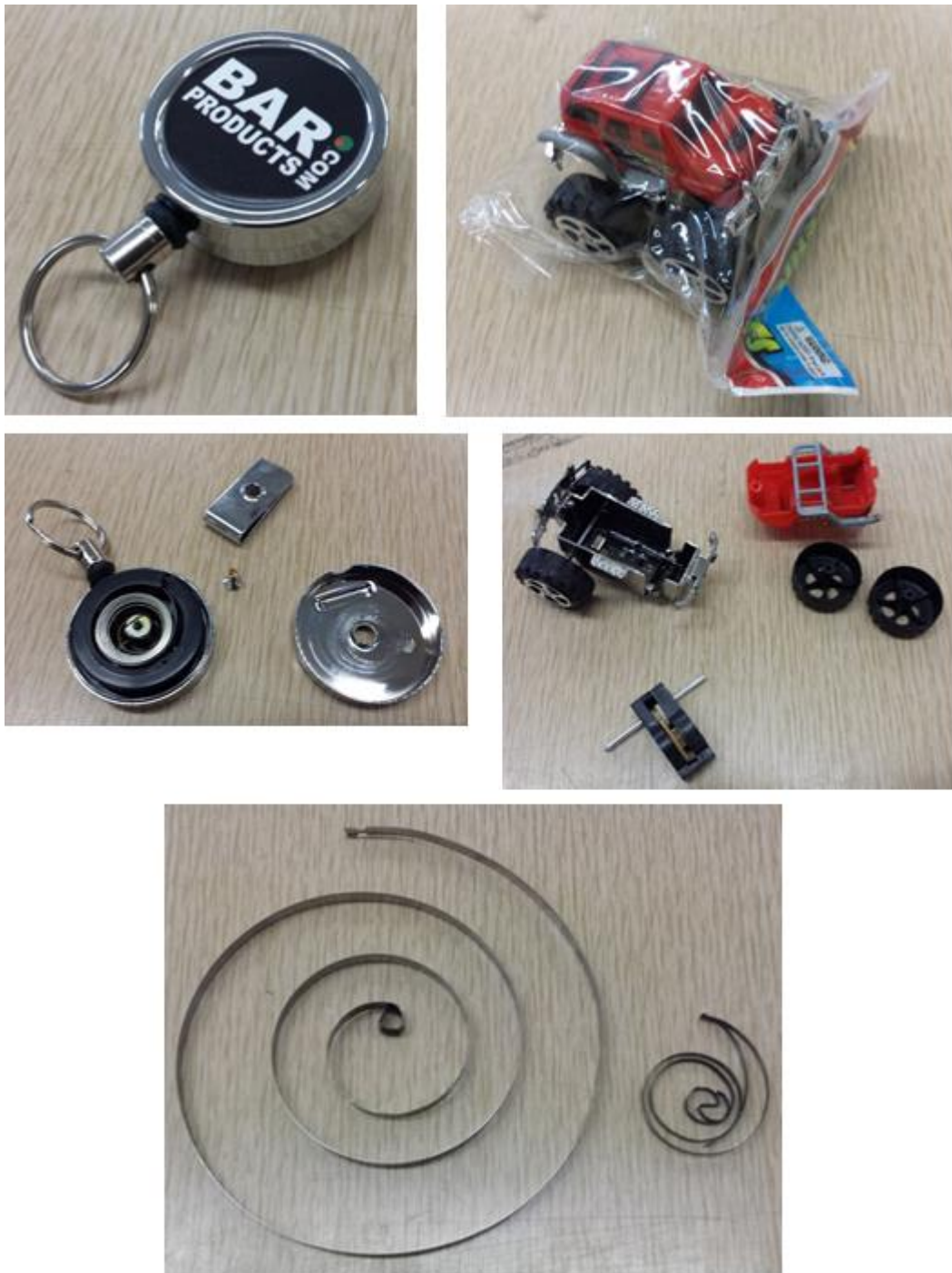
Figure 17: Spring replacement. Left: original spring from reel. Right: spring from a toy car.
