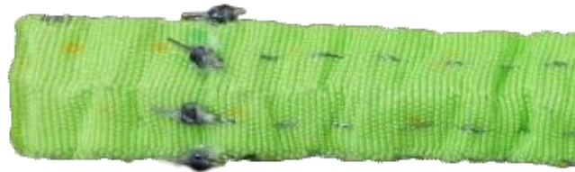
Figure 14: Nylon webbing with conductive thread
