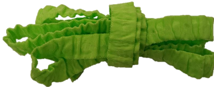
Figure 13: Nylon sheathing removed from hose
