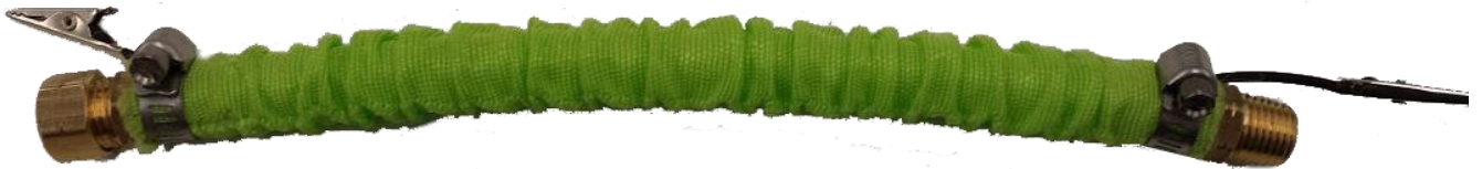
Figure 7: Muscle built using latex, brass fittings, nylon webbing, and conductive rubber
