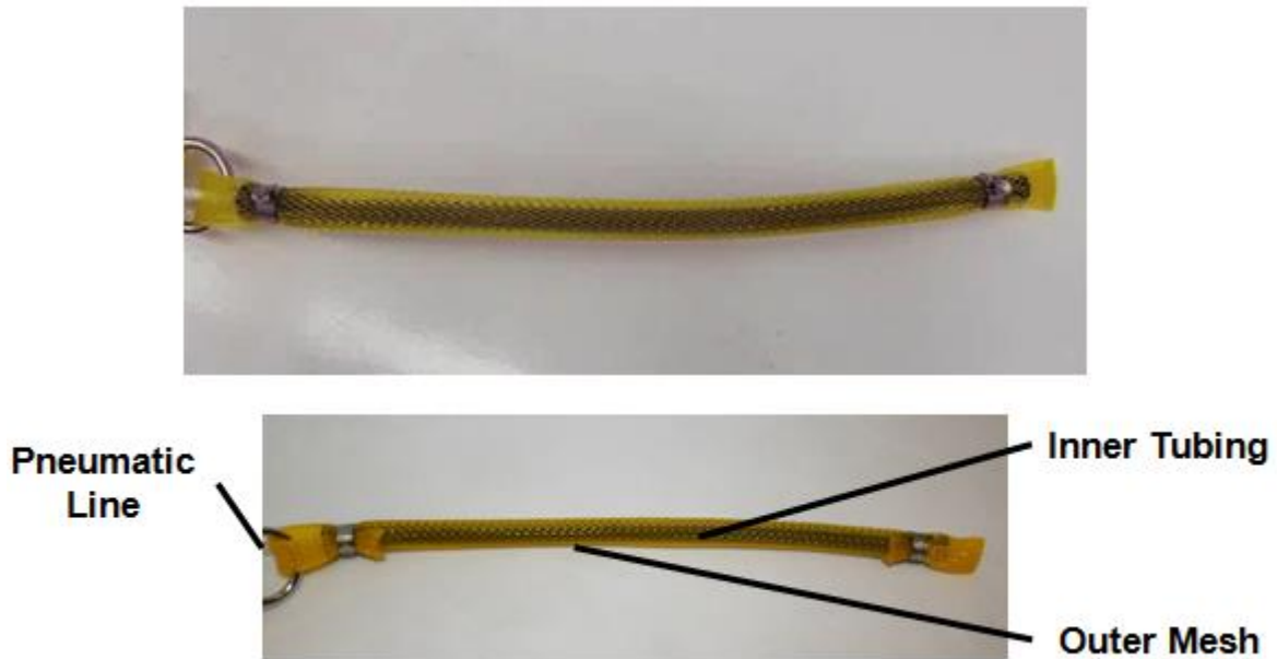
Figure 1: McKibben muscle (“Pneumatic Artificial Muscles”)
