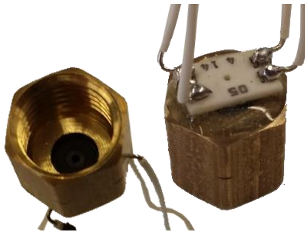
Figure 10: End cap with pressure sensor attached
