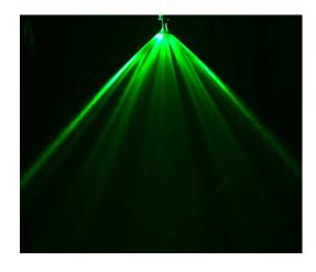
Figure 9: Combined 500 Pictures of 65 Degree Nozzle with 0.1365 m<sup>3</sup>s<sup>1</sup>Pa<sup>-1/2</sup> K-factor at a pressure of 1.38 bar (20 psi)
