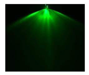
Figure 10: Combined 500 pictures of 125 Degree Nozzle with 0.2277 m<sup>3</sup>s<sup>1</sup>Pa<sup>-1/2</sup> K-factor at a pressure of 1.38 bar (20 psi)
