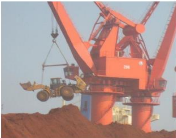
Figure 18: 980H being lifted
