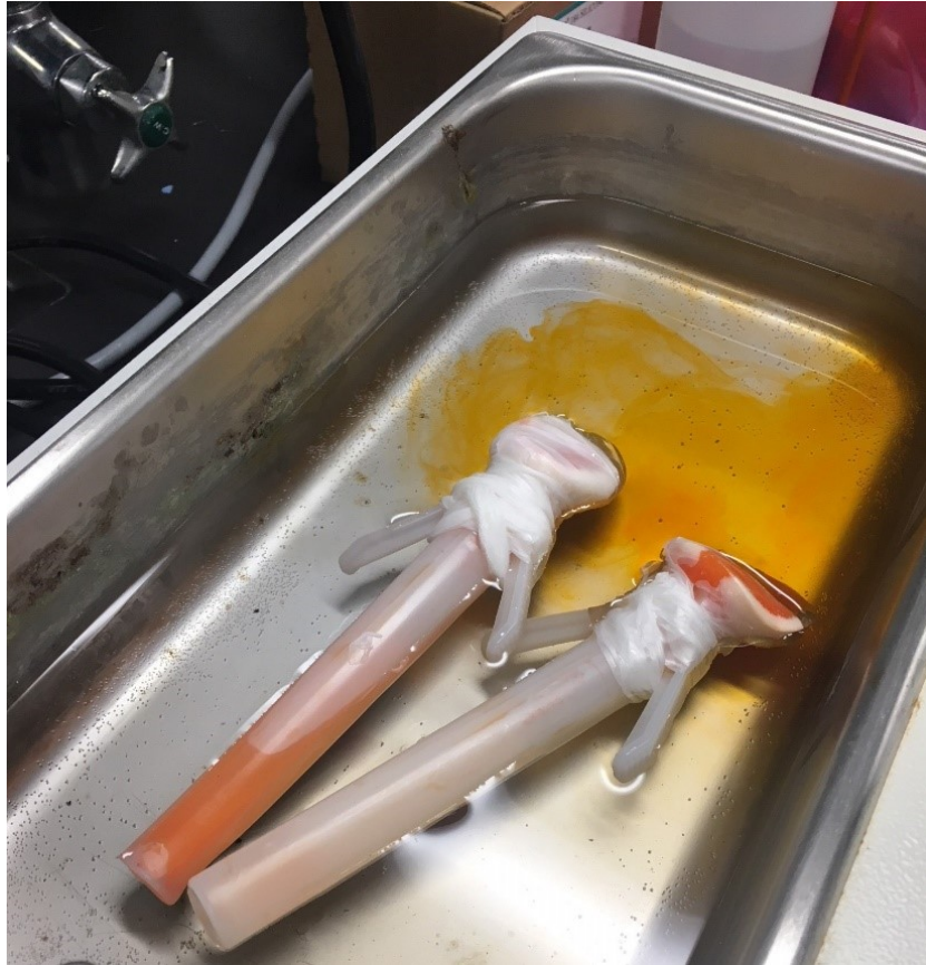
Figure IX. Image of the Chloraprep™ applicators in a water bath at 37°C. After 22 minutes in the water bath, the applicators began to leak orange coloring from their sponge applicator.
