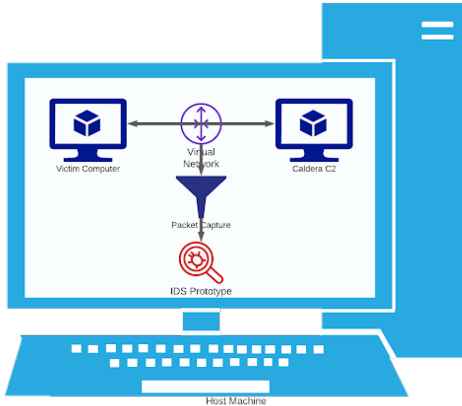
Figure 3.2: Diagram of virtualized network lab environment
