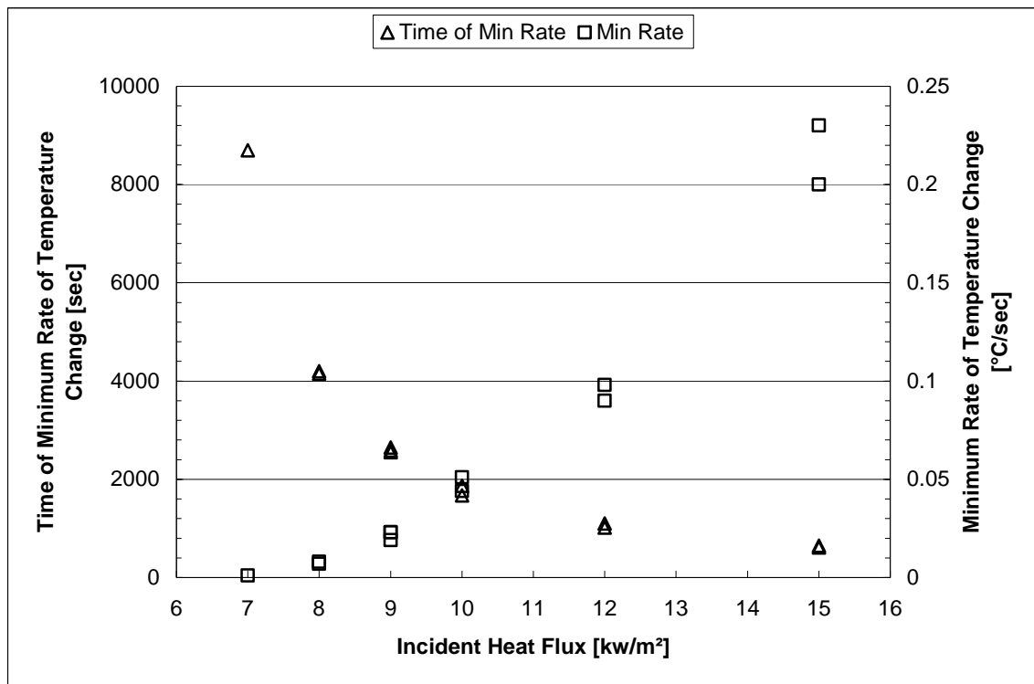
Figure 11 – Co plot of time and rate of minimum rate of temperature change for specimen exposed to heat fluxes between 7 and 15 kW/m 2 .
