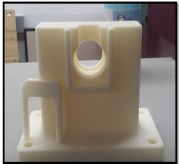
Figure 20: 3D printed mount for a penny-wise speaker
