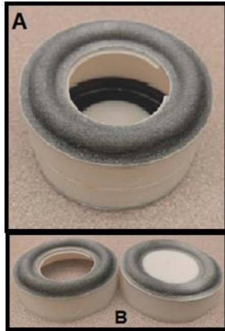
Figure 12: Initial prototype of a dual passive radiator [7]
