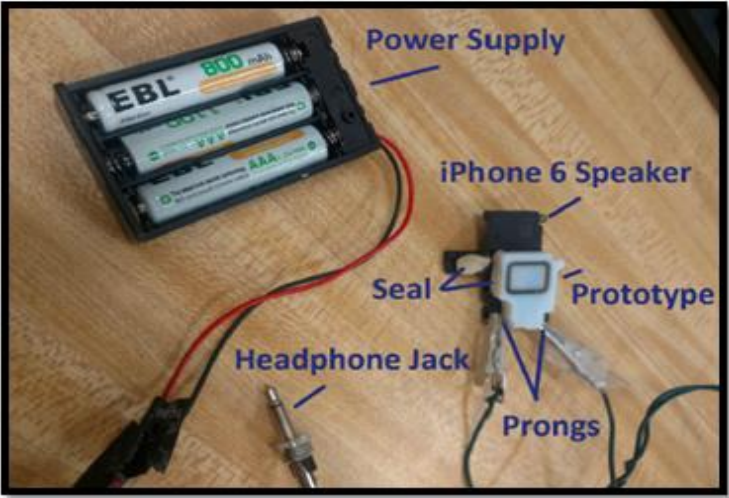
Figure 10: Test set up for recreating an iPhone 6 speaker [7]
