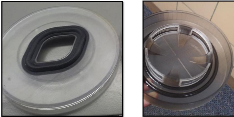
Figure 41: Daffodil Box Design 1 Version 2 3D printed prototype
