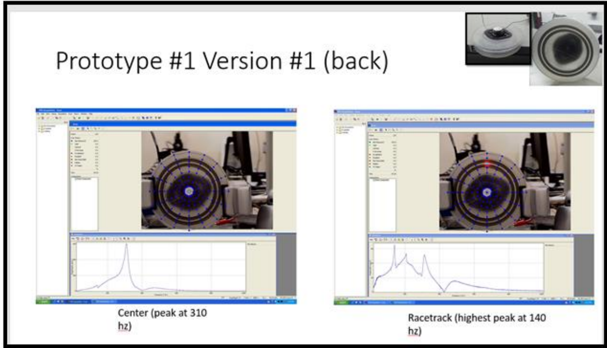
Figure 38: Daffodil Box Design 1 Version 1 Polytec Scanning Vibrometer scans
