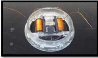
1) Moving Magnet Transducer
