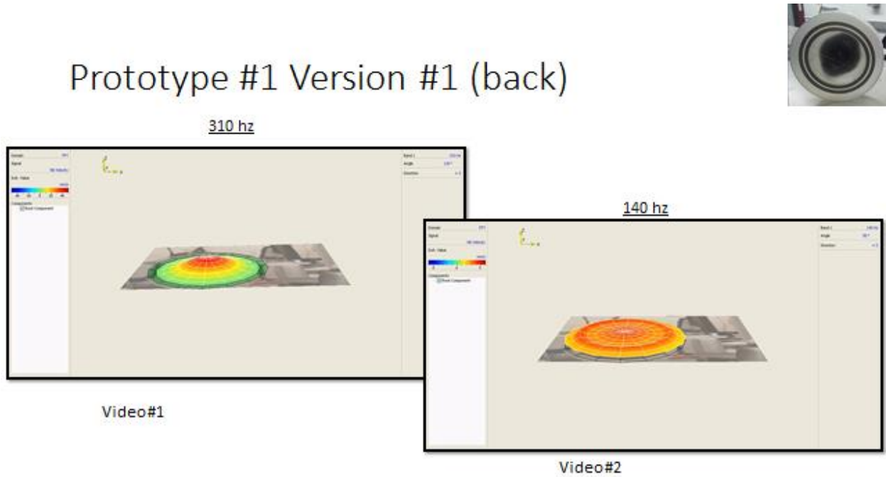
Figure 38: Daffodil Box Design 1 Version 1 Polytec Scanning Vibrometer scans
