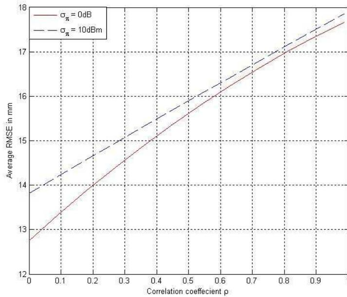
Figure 6.7: The CRLB versus correlation coefficient  $\rho$ , for two different  $\sigma_\pi$  with 64 sensors in parallel configuration. The path loss model parameters are  $\sigma_{dB} = 7.85$  and  $\alpha = 4.26$
