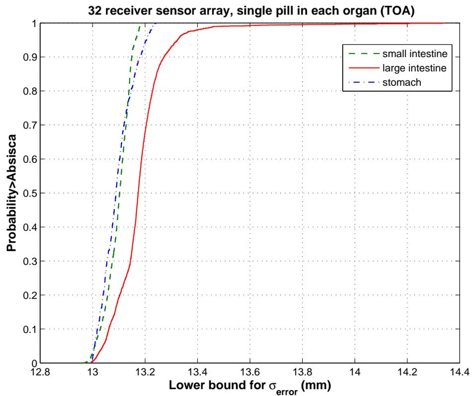
Figure 6.1: The CDF of location error bounds in stomach, small intestine and large
