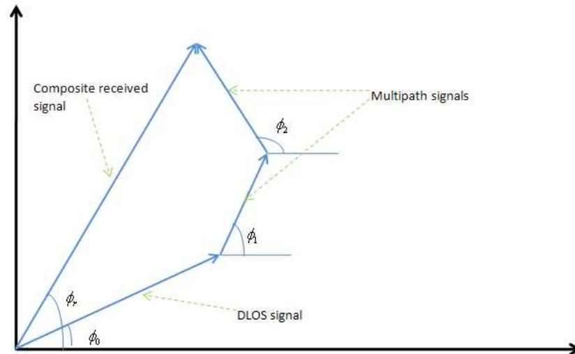
Figure 2.4: Phasor diagram for narrowband signaling on a multipath channel
