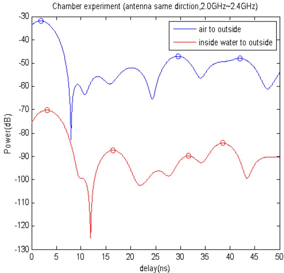
Figure 2.18: Chamber experiment(antenna same direction, 2.0GHz 2.4GHz)
