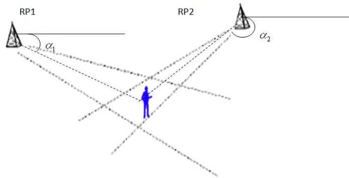
Figure 2.2: AOA technique for geolocation
