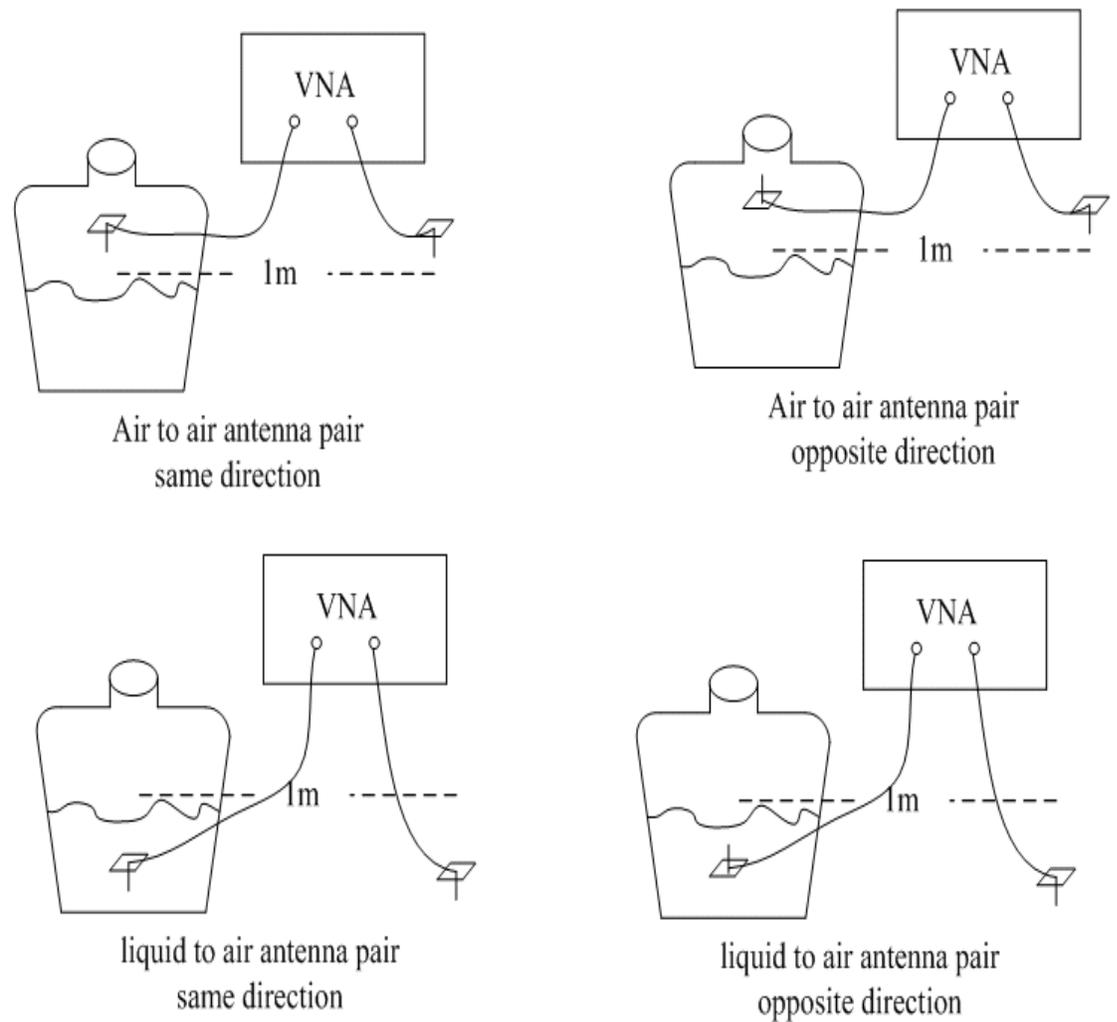
Figure 2.13: Measurement setup
