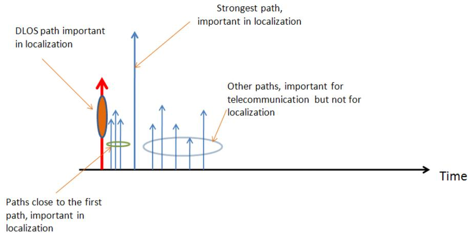
Figure 2.3: Multipath profile and important paths for geolocation
