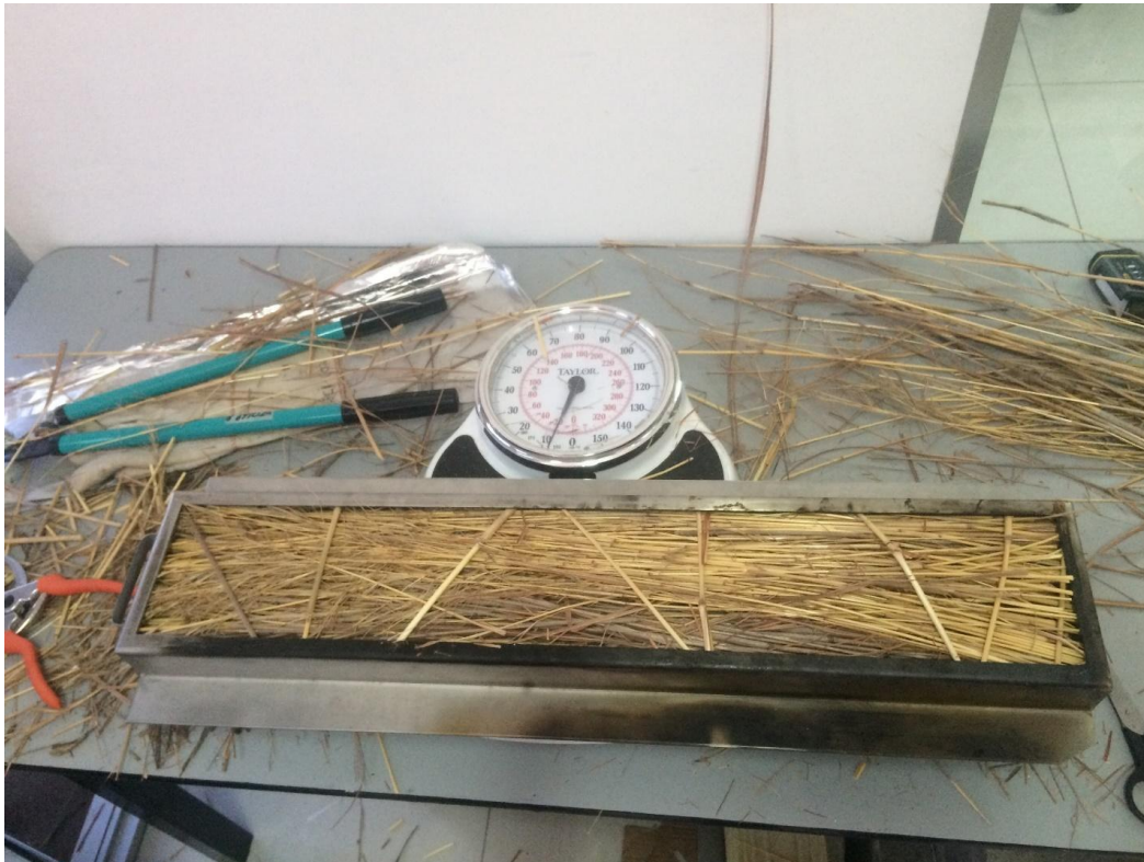
Figure 3.1 Jaragua within Flame Spread Containment Vessel Photograph by Winton Parker
