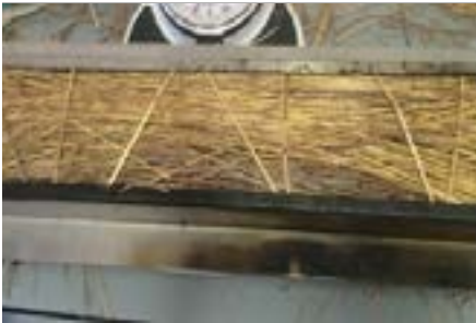
Figure 4. Jaragua in Flame Spread Frame Photographed by Corey Alicchio
