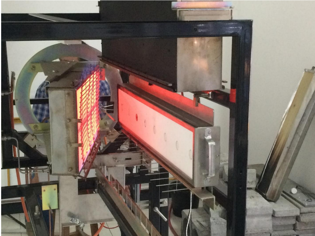
Figure 3.2 Heater Angled 15 Degrees Parallel to Sample Photograph by Authors
