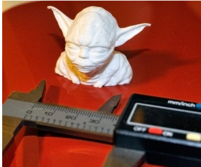
Figure 1.9-4: High resolution Yoda bust printed on a late-model Ultimaker printer with advanced and modified software 20 .
