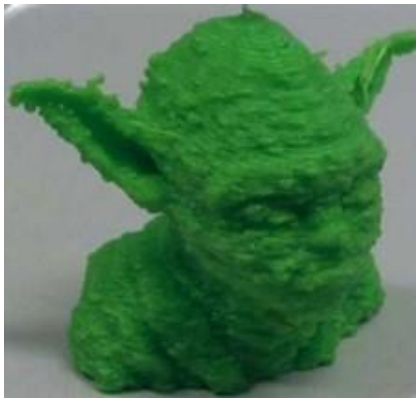
Figure 1.9-3: Low resolution print of Yoda bust test model printed on early model Ultimaker using stock software packages 15 .
