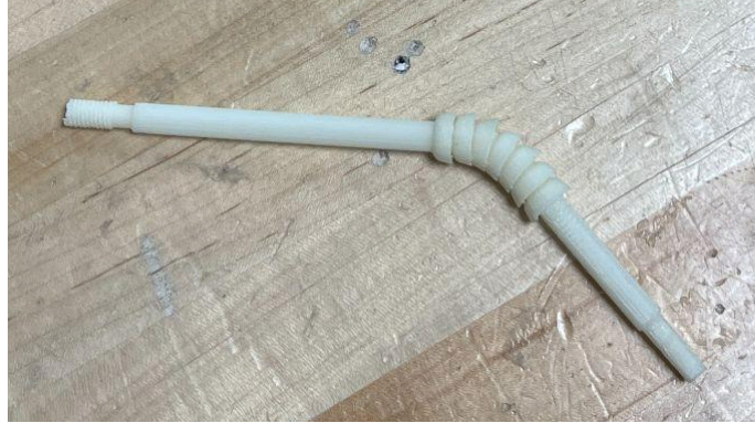
Fig. 27. Bended portion of ABS tubing via heat gun.
