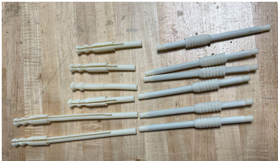
Fig. 22. Tubing Prototype, Final 3D Print in ABS.
