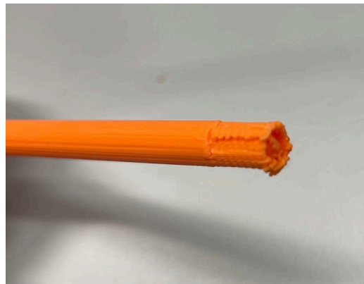
Fig. 24. PLA Tubing Component Threads.
