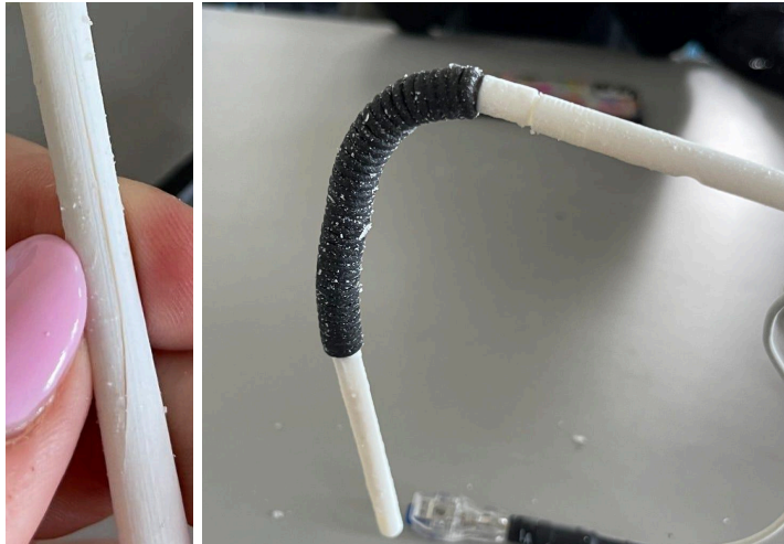
Fig. 25. Tubing Component Material Failure with Vero and Agilus.
