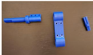
Figure 10: Flex Shaft Couplings
