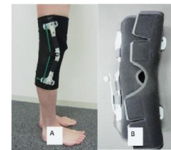
Figure 2: Brace designed by Ota et al which included a charging component about the knee
