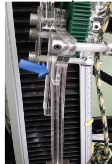
Figure 19: The location of brace failure.
