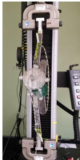
Figure 20: The brace in the fully extension position with relaxed springs.
