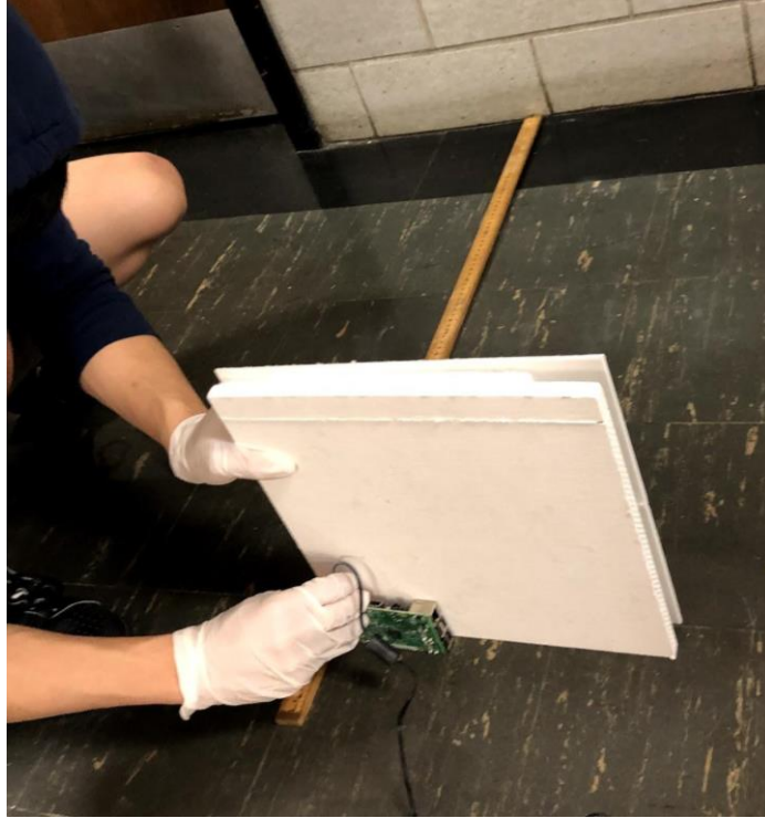
Figure 42: Radar Test Experimental Setup with Insulation.
