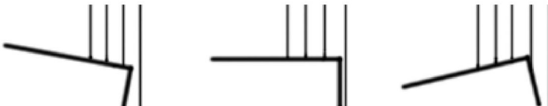
Figure 25. The Behavior of the Laser Sensor Scanning the Edge in Three Different Poses
