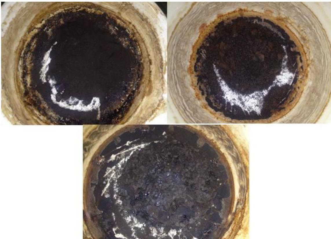
**Figure 14: Bio-char from Three Different Particle Sizes; Top Left 106-150  $\mu\text{m}$ ; Top Right 212-300  $\mu\text{m}$ ; Bottom 1680-2000  $\mu\text{m}$**
