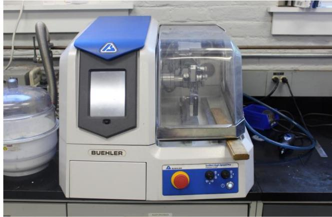
*Figure 63: Buehler metal cutter used in project*
