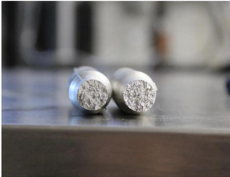
*Figure 43: Results of the third (left) and first (right) iteration tensile tests show the structural differences caused by melting*
