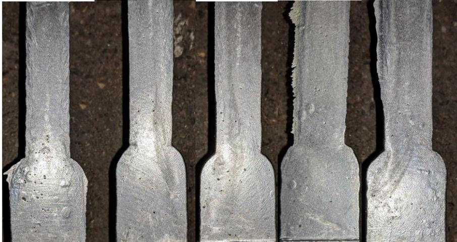
*Figure 48: Hot tearing sample for 3% silicon*
