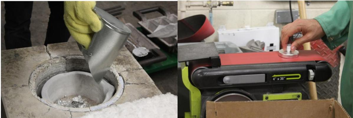
*Figure 53 (Left): Adding metals to melted aluminum*
