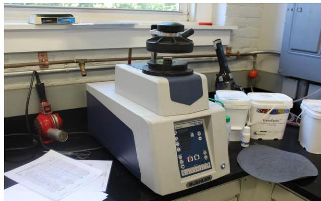
*Figure 64: Buehler resin sample moulder used in project*
