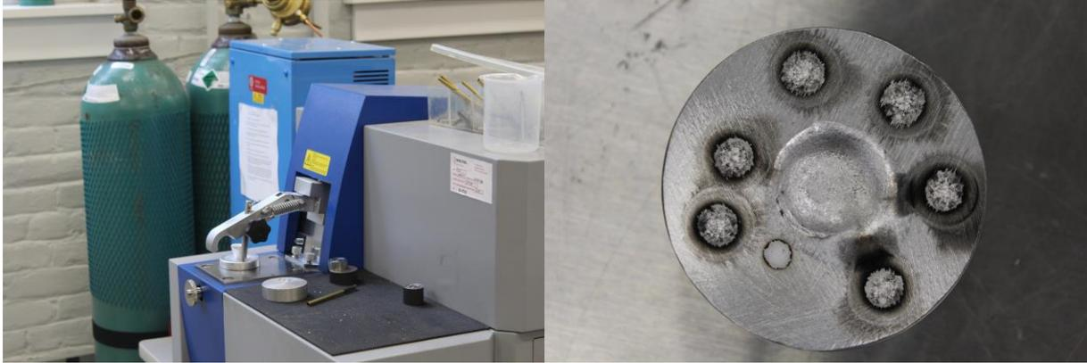
*Figure 55 (Left): Composition testing sample*
