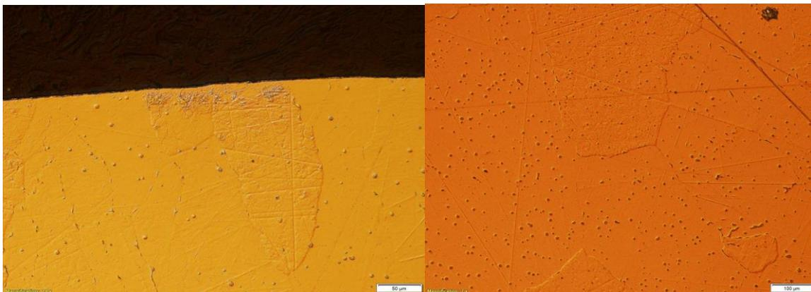
*Figure 23 (Left): 50µm magnification at edge of as cast sample*
