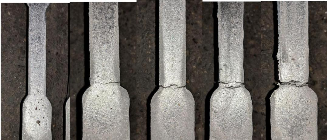
*Figure 46: Hot tearing bars shortest to longest 0% silicon*
