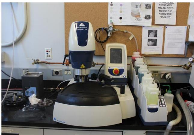
*Figure 65: Buehler polisher used in project*
