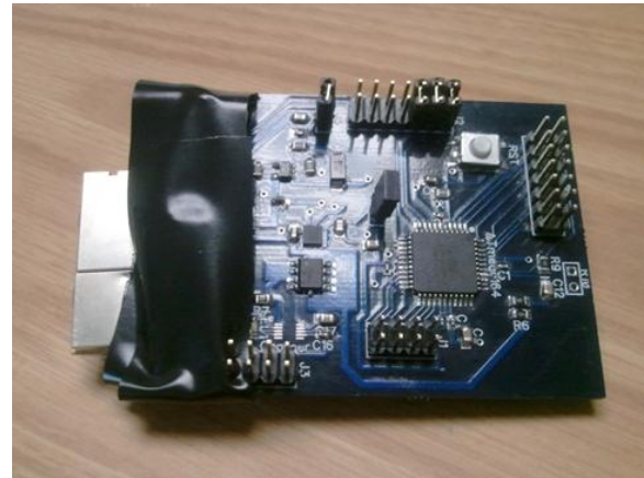
Figure 4-6: Bottom of Victim Unit: CPU & Power Regulation
