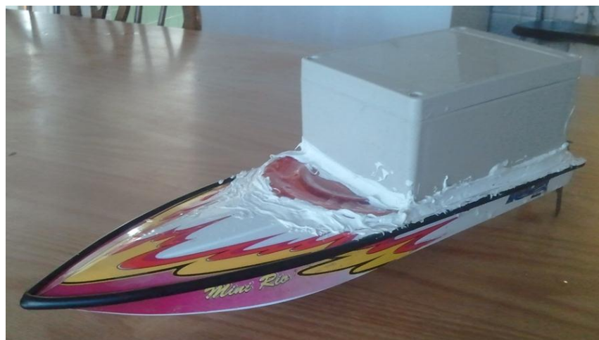
Figure 4-11: Rescue Vehicle with Waterproof Box
