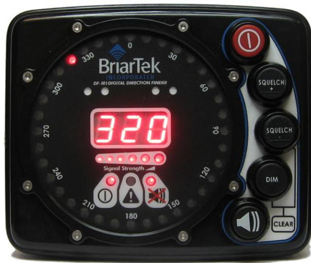
Figure 2-3: ORCA Direction Finder Display Unit 3
