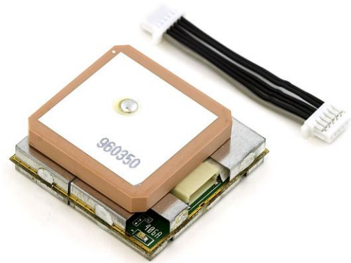
Figure 4-3: EM406a GPS Receiver
