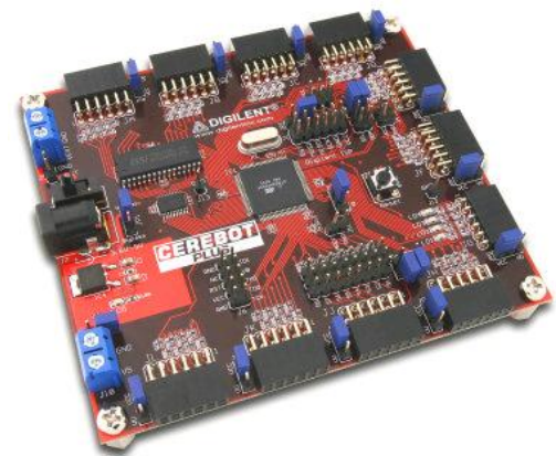
Figure 4-8: Development board: Digilent Cerebot Plus
