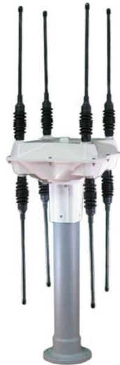
Figure 2-2: ORCA Direction Finder Antenna Array 2
