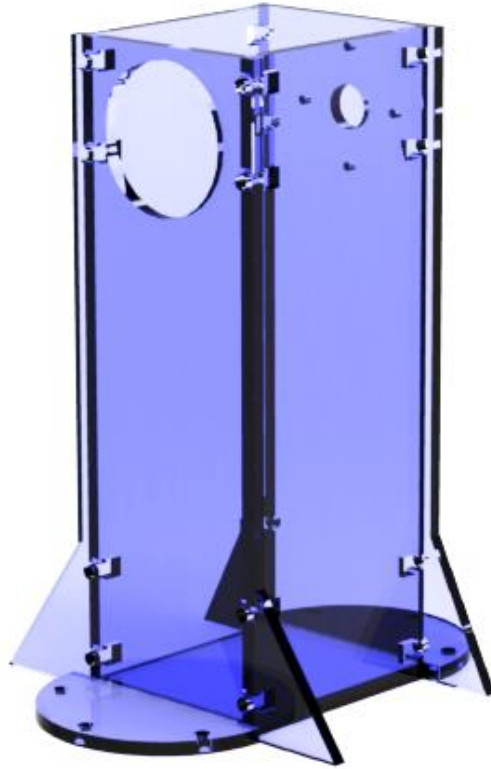
Figure 23. Motor mount fixture for holding the CIM motor
