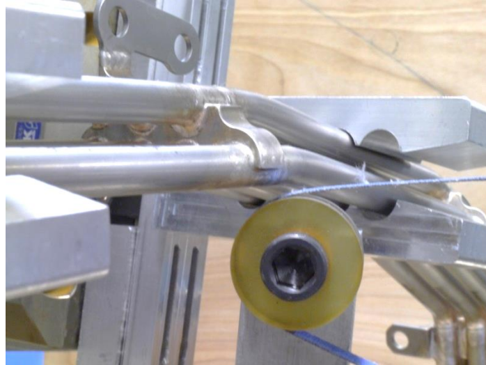
Figure 29. Polishing belt coming into contact with the tube
