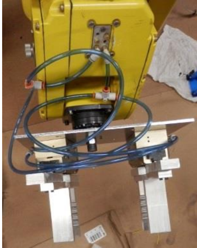
Figure 36. The pneumatic tubing.
